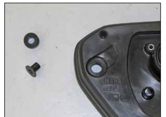
7. Remove the reinforcement and mounting grommet from the back plate as shown.
