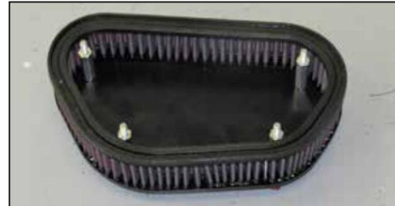
17. Install the K&N® air filter onto the front plate as shown.
