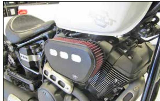
18. Install the front plate and filter assembly onto the back plate and secure to it to the back plate with the provided hardware.
