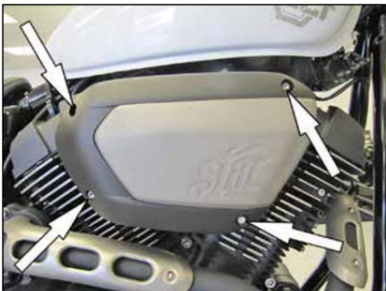
2. Remove the four bolts that secure the cover and filter to the base and then remove the cover and filter from the vehicle.
