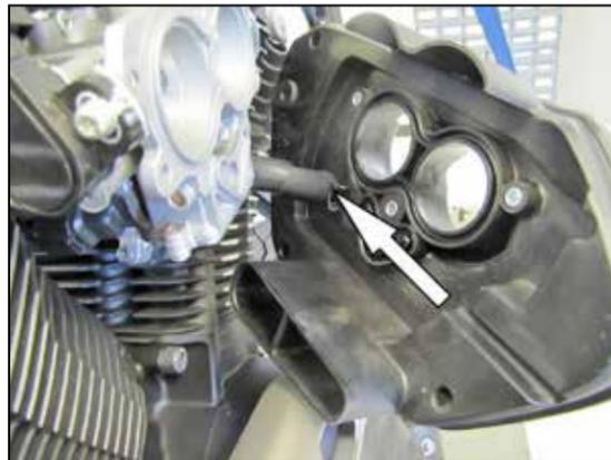
4. Pull the filter base away from the throttle body then release the spring clamp securing the crank case vent hose and disconnect the crank case vent hose from the back plate.
