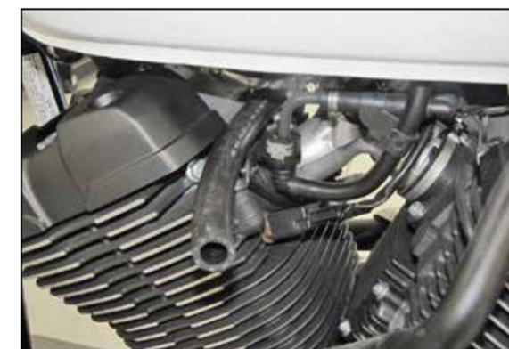
11. Route the provided crank case vent hose on top of the throttle body as shown so that it comes out of the left side of the engine.
