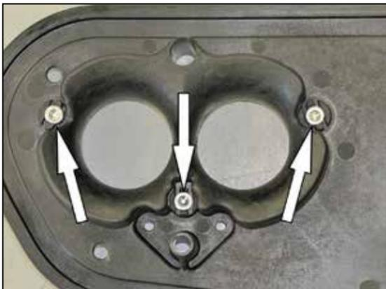
10. Install the factory throttle body bolts into the K&N® back plate as shown.
