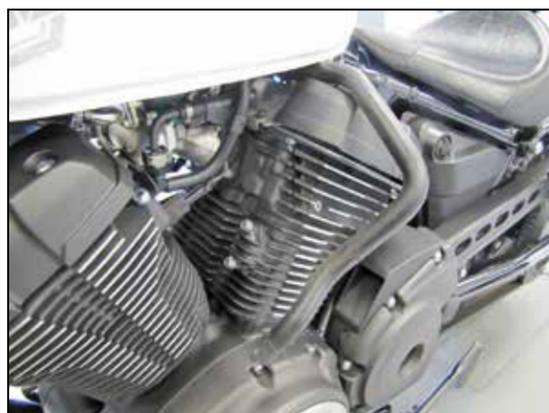
5. From the left side of the vehicle, pull the crank case vent hose out for later access.
