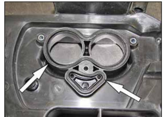
6. With a small screw driver or pick, carefully remove the factory gaskets from the filter back plate.
