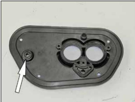
9. Install the factory grommet and reinforcement into the K&N® back plate as shown.
