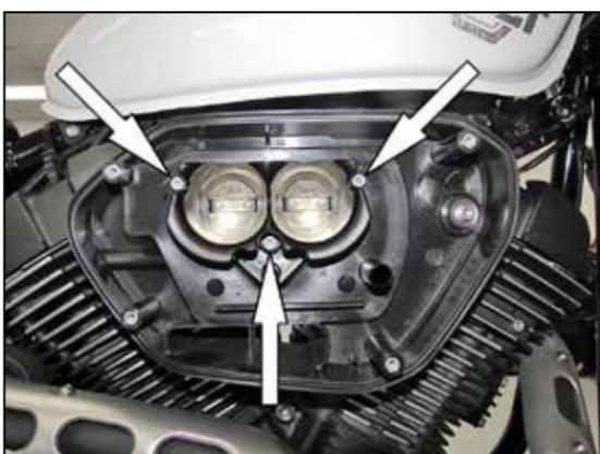
3. Remove the three Throttle body bolts and the mounting bolt shown.
