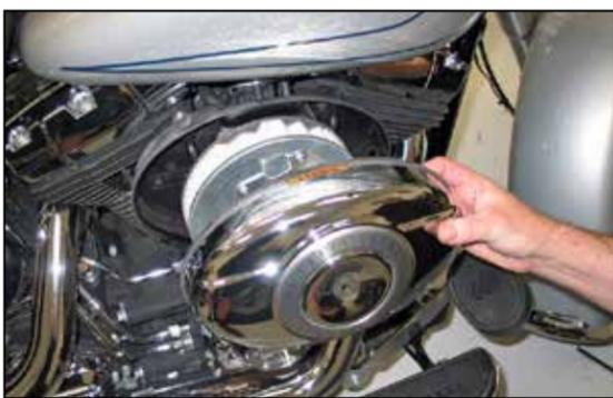
2. Remove the bolt that secures the bonnet to the filter assembly and then remove the bonnet from the vehicle.
