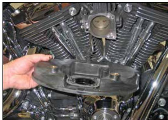
5. Remove the air filter base from the throttle body and unhook the wiring pig tail from the filter base.
