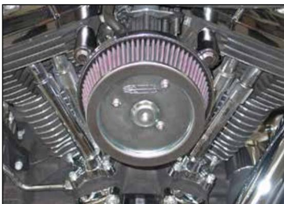
11. Install the K&N® air filter onto the base plate and secure with the provided hardware.
