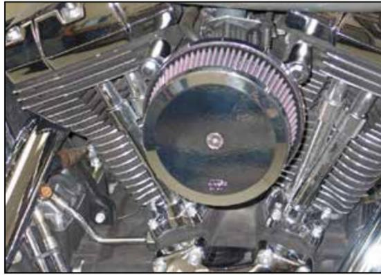
12. Install the filter cover plate onto the K&N® air filter and secure with the provided hardware.
