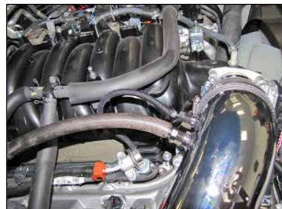
21. Install the crank case hose assembly into the factory crank case vent, Then connect the crank case vent hose and the fuel pressure hose to the fittings installed into the K&N® intake tube.
