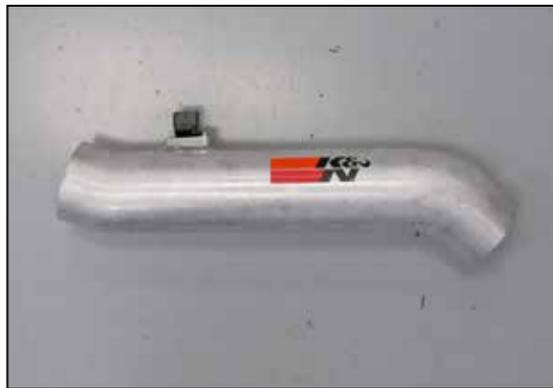
13. Install the mass air sensor into the K&N intake tube and secure with the provided hardware.
