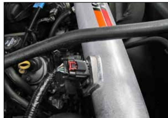
20. Reconnect the mass air sensor electrical connections.
