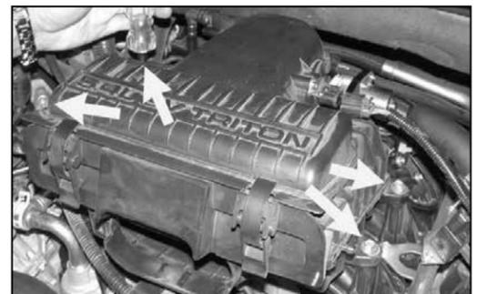
7. Remove the four bolts that secure the air cleaner as shown.
