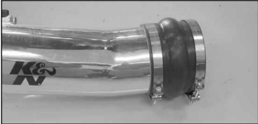
19. Install the silicone hose and hose clamps onto the K&N® intake tube as shown.
