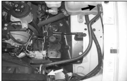
15a. Loosen the coolant recovery hose, hose clamps, and then remove the factory recovery hose shown. Be sure to catch any coolant, which flows out of the radiator during hose removal.
