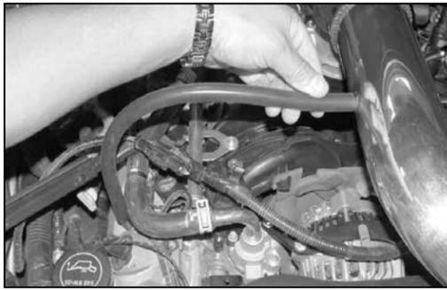
23. Install the provided silicone hose onto the vent on the cam cover, then, connect the other end to the vent on the K&N® intake tube as shown.
