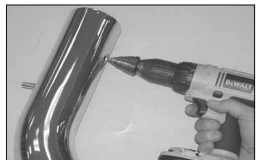
17b. Remove the intake tube and drill a 5/8" hole at the location marked in step #17a.
