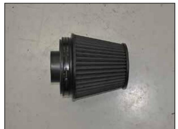
21. Install the filter adapter into the K&N® air filter and secure with the provided hardware.
