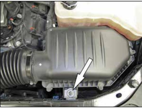
7. Remove the bolt which secures the air filter housing to the core support and then remove the complete air filter system from the vehicle.
