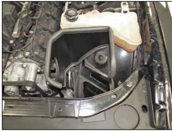
12. Install the heat shield into the vehicle and secure with the provided hardware.
