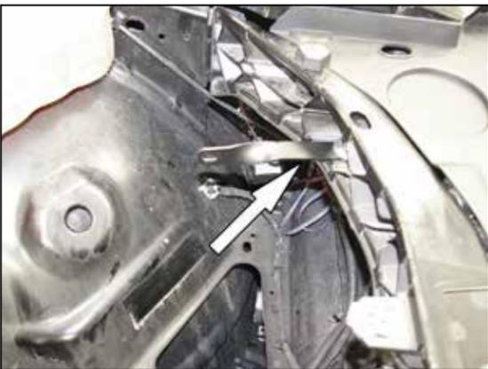
9. Install the heat shield mounting bracket (070772) onto the core support using the provided hardware.
