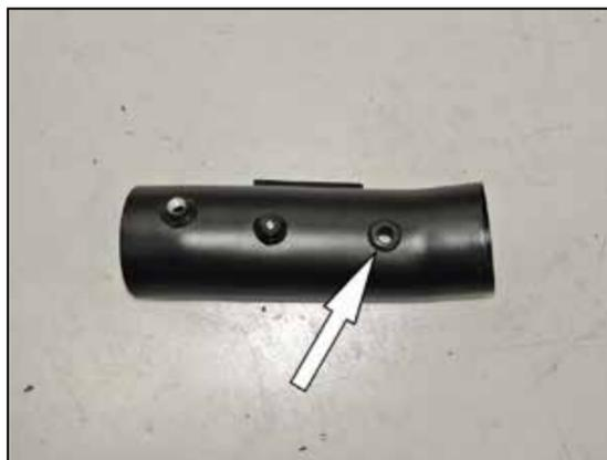
16. Using the provided grommet, Install the inlet air temperature sensor into the K&N® intake tube,
