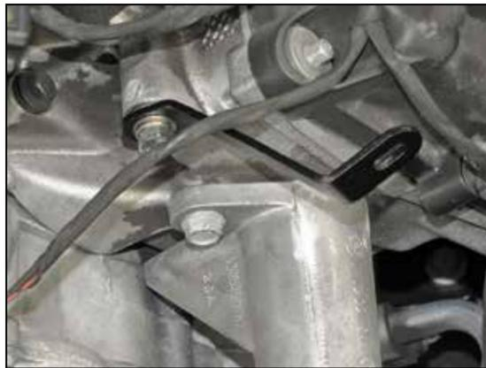
13. Install the tube mounting bracket (010088) onto the cylinder head as shown. Be sure to place the provided spacer between the bracket and cylinder heads.
