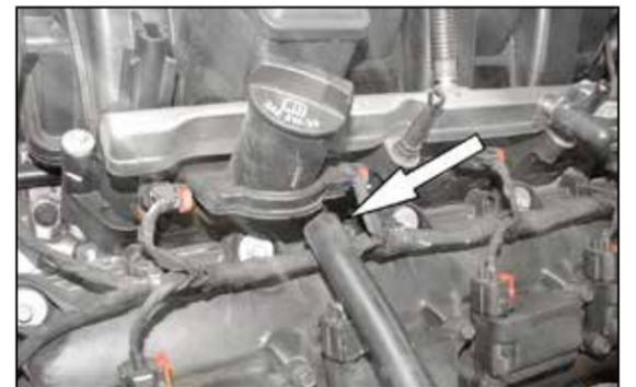
5. On models equipped with a 5.7L. Disconnect the crank case vent hose from the valve cover port.
