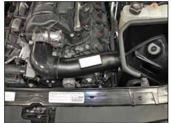
18. Install the K&N® intake tube into the silicone hose and align with the mounting bracket installed earlier. Secure with the provided hardware and hose clamp.
