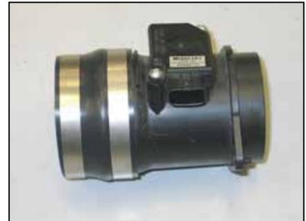
24. Install the provided silicone hose (084031) onto the mass air sensor and secure with the provided hose clamp.
