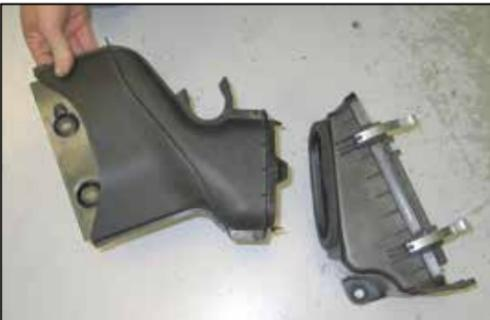
14. Open the air box halves and then push the fresh air intake scoop out of the front air box half.
