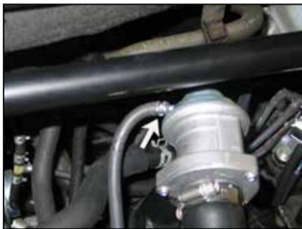
5. Release the spring clamp that secures the bypass valve signal line and then disconnect the bypass valve signal line from the bypass valve.
