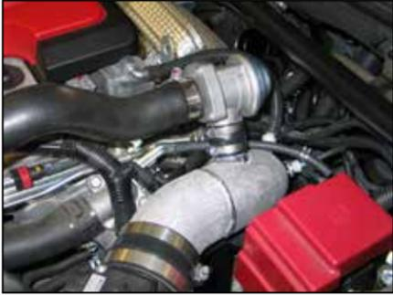
29. Install the bypass valve with silicone hose onto the K&N® intake tube and secure with the provided hose clamp.
