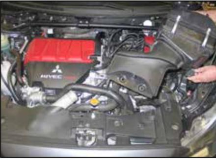
10. Remove the complete air box assembly from the vehicle.
