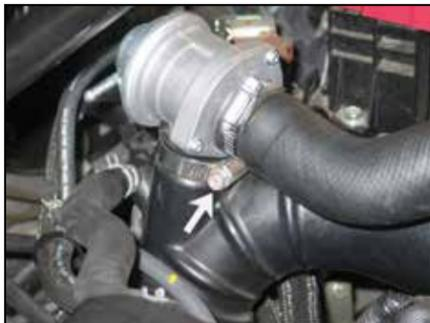
6. Loosen the hose clamp securing the bypass valve to the intake tube and then disconnect the bypass valve from the intake tube, set it to the side.
