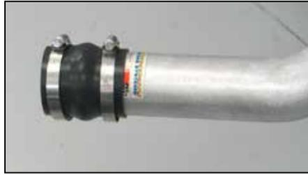
32. Install the remaining silicone hose (08487) onto the K&N® upper intercooler tube as shown, slide the hose completely onto the tube and do not secure at this time.
