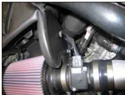
35. Clip the mass air wiring harness onto the heat shield and then reconnect the mass air sensor electrical connection.
