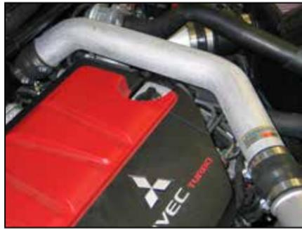
33. Install the K&N® upper intercooler tube into the silicone hose on the turbo outlet, align with the intercooler inlet, slide the silicone hose onto the inlet and then secure with the provided hose clamps.
