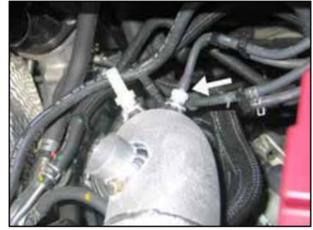
22. Connect the factory vacuum line to the 1/4 NPT fitting as shown.
