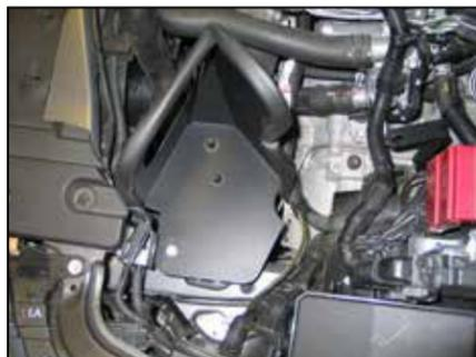
20. Install the heat shield assembly onto the factory air box mounting location and secure with the hardware provided.
