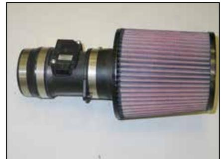
25. Install the K&N® filter onto the mass air sensor and secure with the provided hose clamp.
