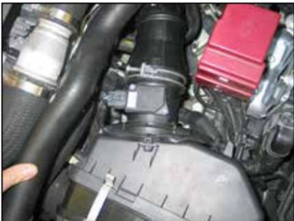
2. Disconnect the mass air sensor electrical connection and unhook the wiring harness from the air box mounting locations.
