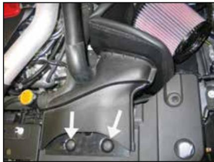
34. Install the fresh air intake scoop into the heat shield as shown and then secure with the factory retaining clips.
