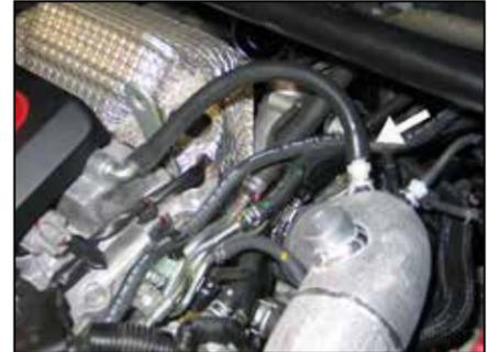
23. Connect the provided crank case vent hose to the remaining 1/4 NPT fitting and then to the valve cover port as shown.
