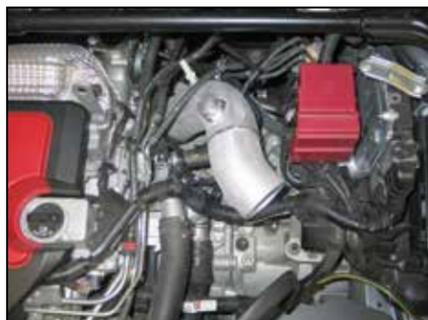
21. Install the K&N® intake tube onto the turbo inlet and align with the mounting bracket installed in step #15. Secure the intake tube with the provided hose clamp and hardware.
