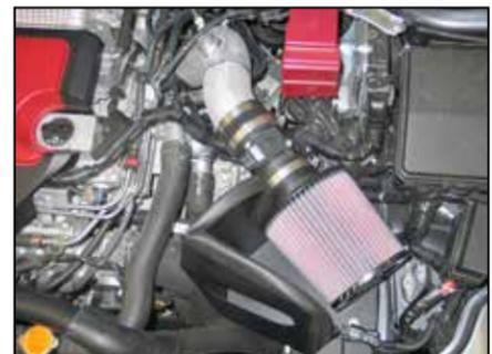
26. Install the mass air sensor assembly onto the K&N® intake tube and secure with the provided hose clamp.
