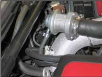
30. Reconnect the factory vacuum hose to the bypass valve and secure with the factory hose clamp.
