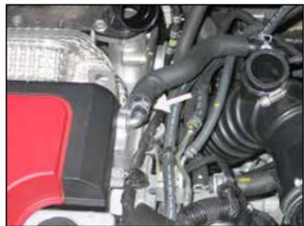
7. Loosen the spring clamp which secures the crank case vent hose to the valve cover and then disconnect the crank case vent hose from the valve cover.
