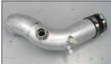
17. Install the silicone hose (084036) onto the K&N® intake tube as shown and secure with the provided hose clamp.
