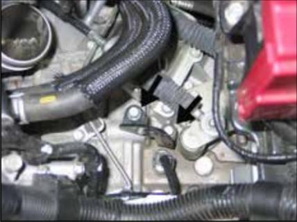
11. Remove the two bolts which secure the transmission/engine lifting bracket and remove the engine lifting bracket from the transmission.
