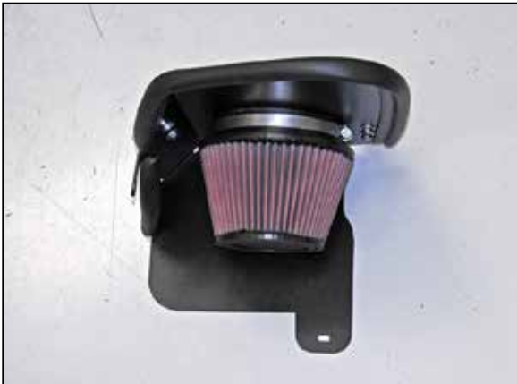
10. Install the K&N® air filter onto the filter adapter and secure with the provided hose clamp. NOTE: Drycharger® air filter wrap; part # RU-5163DK is available to purchase separately. To learn more about Drycharger® filter wraps or look up color availability please visit http://www.knfilters.com .
