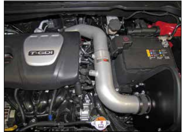
19. Install the intake tube assembly into the coupling hoses, align for best fit and then secure with the provided hose clamps.
