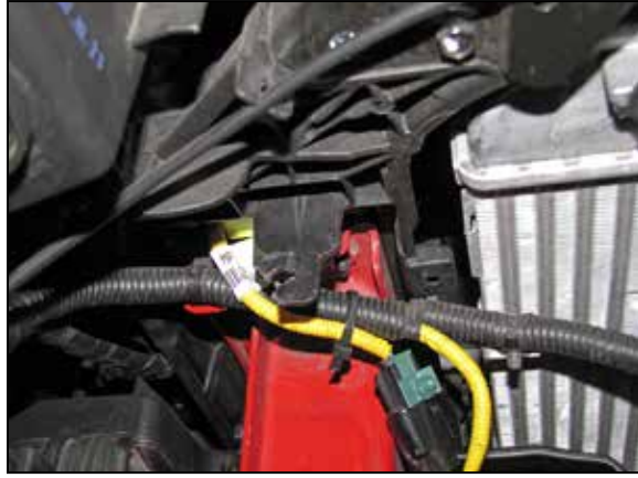
13. Using the provided tie wrap secure the pigtail to the wiring harness below.
