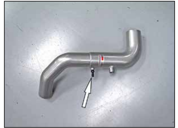
18. Install the provided vent fitting into the K&N® intake tube. NOTE: Plastic NPT fittings are easy to cross thread. Install the vent fitting "hand" tight, then turn it two complete turns with a wrench.
