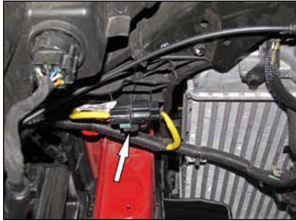
12. Unclip the wiring harness shown from its mounting location.
