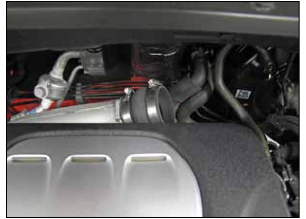
17. Install the provided hump coupler (08185) onto the turbo inlet and secure with the provided hose clamp.
