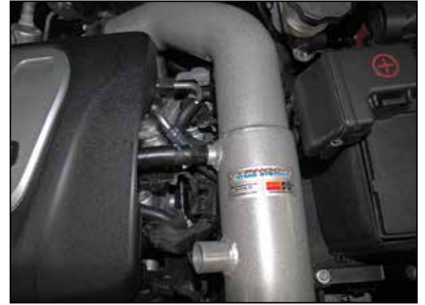
20. Connect the crank case vent hose to the fitting installed into the intake tube and secure with the factory spring clamp.
