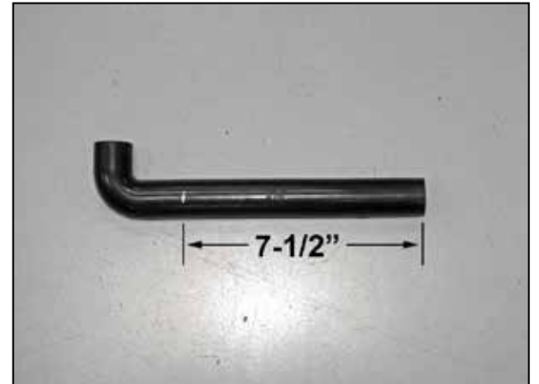
21. Mark and cut the provided BOV hose 7-1/2" from the end. The 7-1/2" section will not be used.
