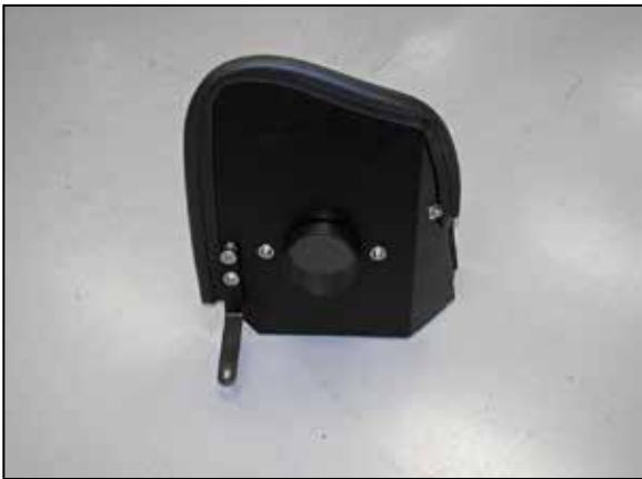
9. Install the filter adapter into the heat shield and secure with the provided hardware.
