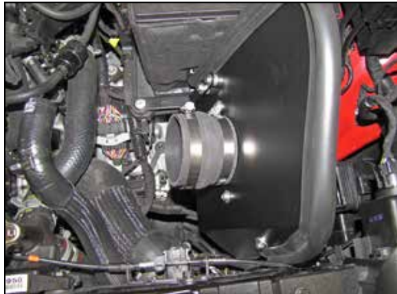
16. Install the provided hump coupler (087121) onto the filter adapter and secure with the provided hose clamp.
