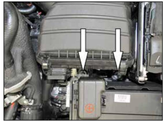
5. Remove the two bolts securing the air box to the mounting bracket. Then remove the air box from the vehicle.
