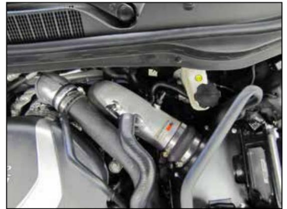
18. Align the intake tube with the filter adapter and slide the silicone hose onto the adapter. Tighten all of the hose clamps for the upper and lower silicone hoses securing the intake tube.
