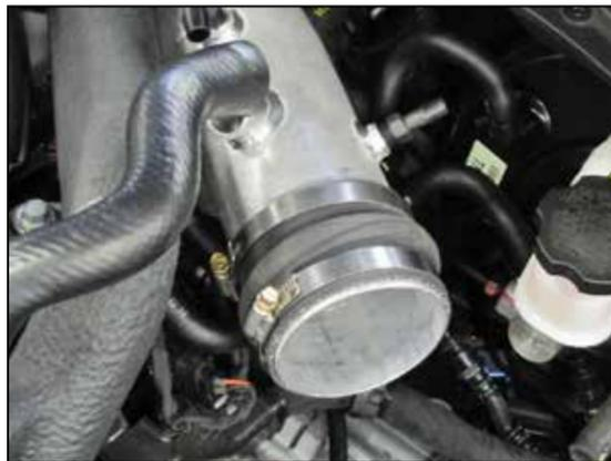
16. Slide the silicone hose (08699) onto the intake tube all the way on. Do not tighten at this time.
