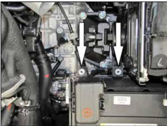
10. Install the two 1/2" high rubber mounted studs provided into the air box mount bolt locations.
