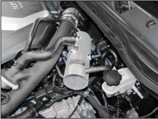
9. Set the K&N® intake tube into position in the silicone hose; do not completely tighten the hose clamp at this time.
