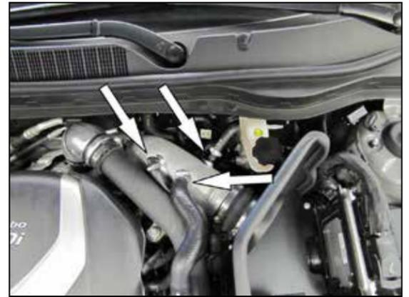
19. Connect the Blow of valve hose, EVAP hose and crank case vent hose to the intake tube and secure with the provided hose clamps.
