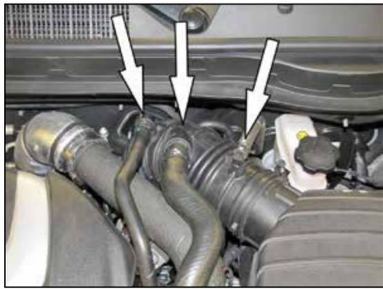
3. Loosen the spring clamps and then disconnect the Blow off valve hose, EVAP hose and Crank case vent hose from the intake tube.
