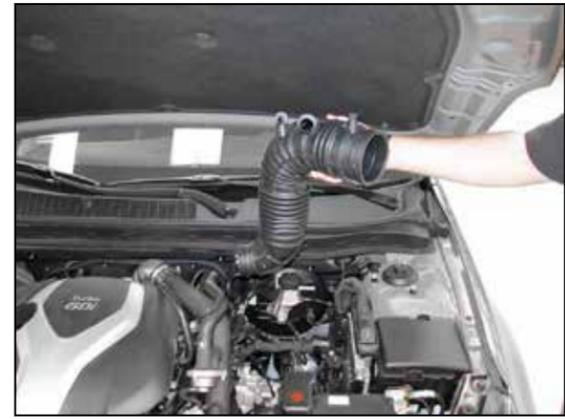
6. Loosen the hose clamp securing the intake tube to the turbo inlet and then remove the intake hose from the vehicle.
