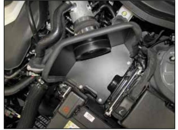
17. Set the heat shield into position on the rubber mounted studs and secure with the provided hardware.
