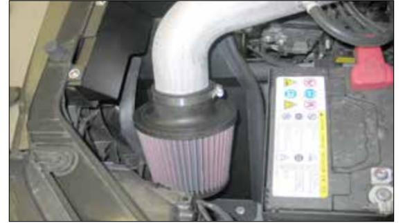
20. Install the K&N® air filter onto the intake tube and secure with the provided hose clamp.
