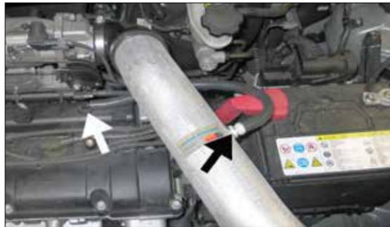
19. Install the provided crank case vent hose onto the 1/4" npt fitting in the K&N® intake tube and then attach the open end to the vent port on the valve cover.
