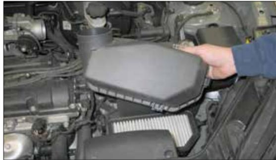
5. Release the upper air box retaining clips and then remove the upper air box from the vehicle.
