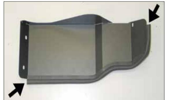
9. Install the 23" long piece of edge trim onto the heat shield as shown.
