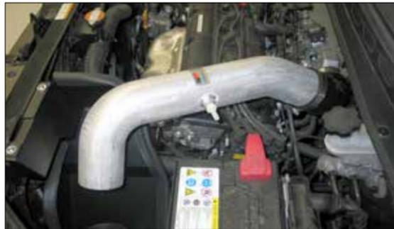
18. Install the K&N® intake tube into the silicone hose at the throttle body and align with the tube mounting bracket. Secure the intake tube with the hose clamp and hardware provided.
