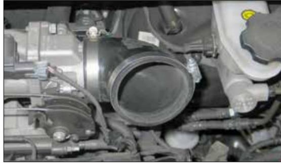
15. Install the provided silicone hose (084087) onto the throttle body and secure with the provided hose clamp.
