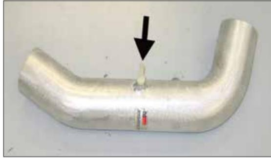
16. Install the provided 1/4npt fitting into the K&N® intake tube as shown.
