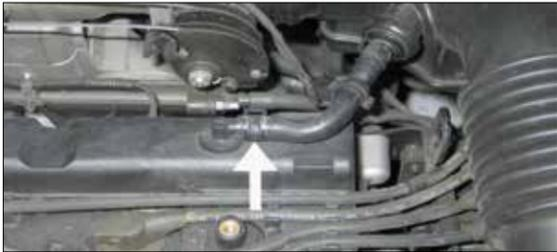
2. Release the spring clamp which secures the crank case vent hose to the valve cover and then unhook the crank case vent hose from valve cover and disconnect the ISC motor wiring harness from the retaining clip attached to the crank case vent hose.
