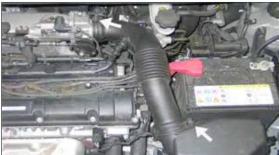
3. Loosen the hose clamps which secure the stock intake tube to the throttle body and air filter housing.
