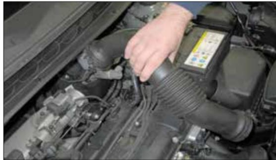
4. Remove the stock intake tube from the vehicle.
