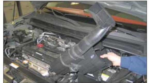
7. Remove the lower air box housing from the vehicle.
