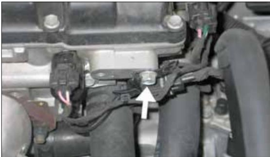
13. Remove the wiring harness retaining bracket bolt shown.
