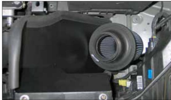
17. Set the K&N® air filter into position at the bottom of the heat shield as shown.
