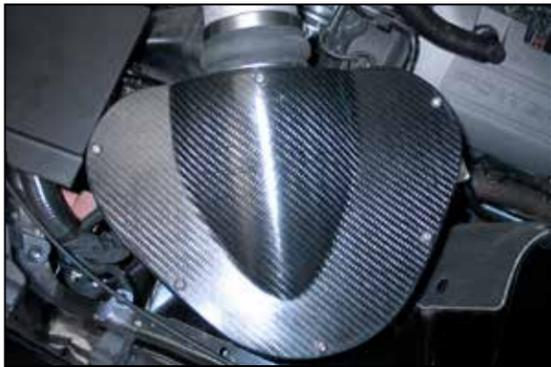
27. Install the K&N® air box lid and secure with the provided hardware.
