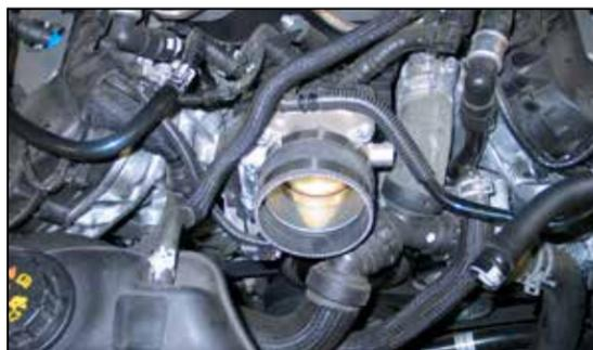
19. Install the provided silicone hose (08698) onto the throttle body and secure with the provided hose clamp.
