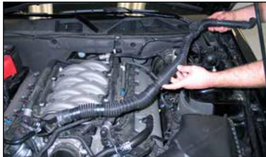
4. Release the clamp that secures engine pulse hose to the intake tube, then remove the engine pulse hose from the vehicle.
