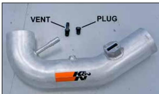
20. On vehicles that have an EVAP vent line attached to the intake tube, install the 3/8" vent fitting into the K&N® intake tube. On vehicles that do not have the EVAP vent line attached to the intake tube, install the npt plug into the intake tube.
