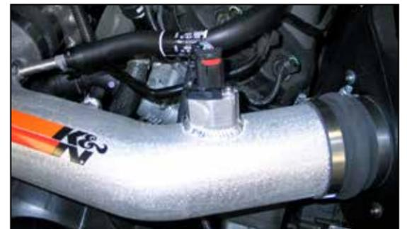
25. Reconnect the mass air sensor electrical connection.
