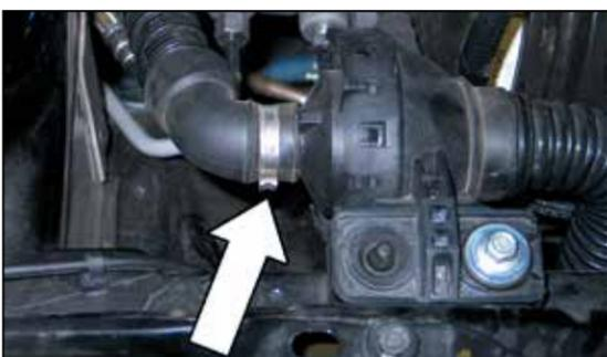
3. Cut the clamp that secures the engine pulse hose to the drum and disconnect the hose from the drum.
