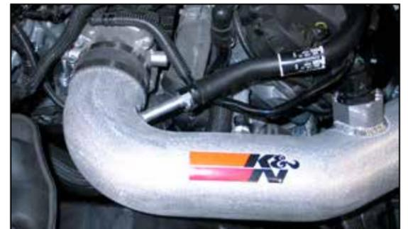
24. Connect the crank case vent hose to the fitting on the K&N® intake tube.
