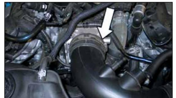
8. Loosen the hose clamp that secures the factory intake tube to the throttle body.
