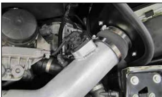
17. Connect the crank case vent hose to the fitting installed into the K&N intake tube and reconnect the mass air sensor electrical connection.
