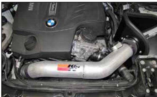
16. Install the K&N intake tube into the factory turbo inlet tube and then into the filter adapter coupler hose. Adjust the tube and heat shield for best fit and then secure the hose clamps and heat shield hardware.
