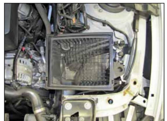
6. Lift up and remove the lower air filter housing from the inner fender.
