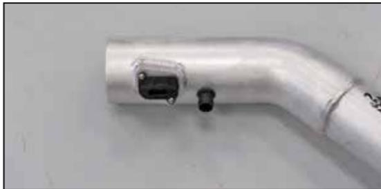
15. Install the mass air sensor into the K&N intake tube and secure with the provided hardware.
