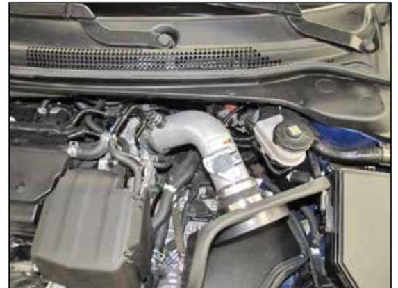
20. Install the K&N® intake tube into the coupling hoses and adjust the tube for best fit then secure with the provided hose clamps.
