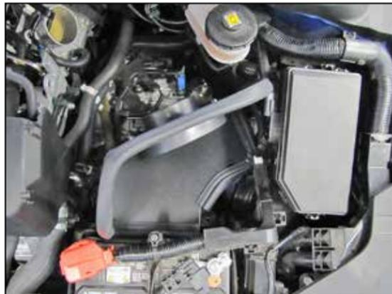
15. Install the heat shield into the vehicle so that the grommet slides onto the mounting stud and the front lines up with the rubber mounted studs. Secure the heat shield with the provided hardware and secure the transmission vent line to the clip installed into the heat shield.
