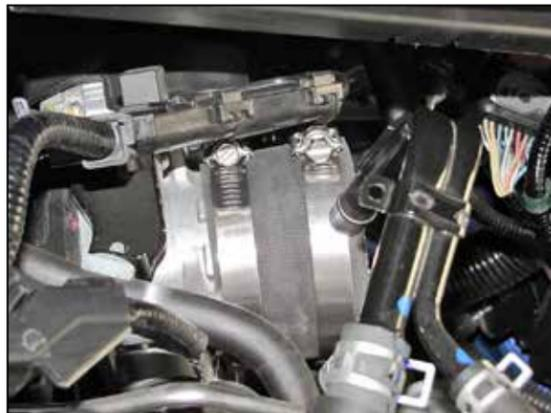
16. Install the provided coupler (08440) onto the throttle body and secure with the provided hose clamp.
