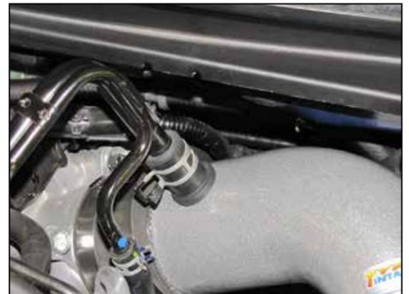
21. Insert the crankcase vent tube into the grommet installed into the K&N® intake tube and use the factory spring clamp to secure. **NOTE: It is designed to be a snug fit to prevent any possible crank case vent leaks.**
