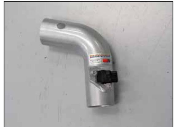
18. Remove the mass air sensor from the factory air filter housing and install it into the K&N® intake tube using the provided hardware.
