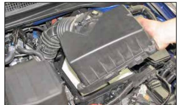
5. Lift up and remove the upper air filter housing and remove it from the vehicle.
