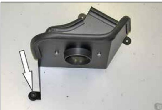
11. Remove the factory air filter housing mounting grommet from the factory air filter housing and install it into the K&N® heat shield as shown.
