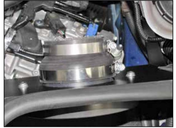
17. Install the provided step coupler (084093) onto the filter adapter and secure with the provided hose clamp.
