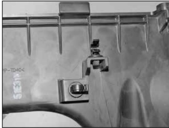
13. Remove one of the transmission vent hose clips from the lower air filter housing.
