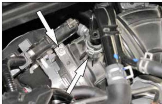
3. Release the spring clamp securing the crank case breather tube and then loosen the hose clamp that secures the intake tube to the throttle body.
