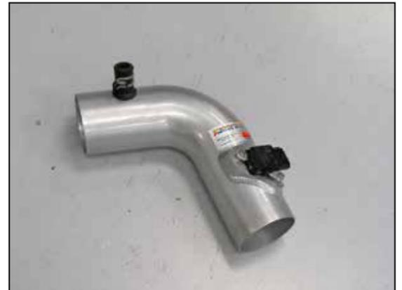
19. Install the provided grommet into the K&N® intake tube along with the factory crank case vent spring clamp.
