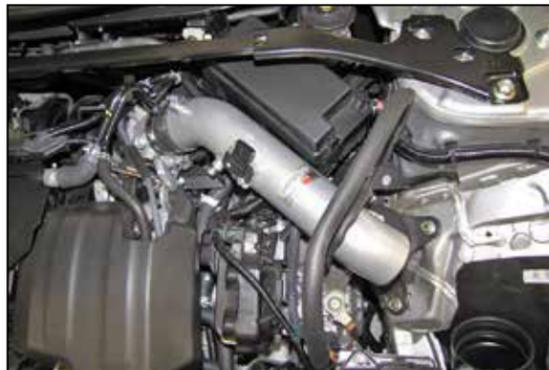
15. Install the K&N® intake tube through the heat shield, into the silicone hose at the throttle body and align with the mounting bracket. Secure the tube with the provided hardware and hose clamp.
