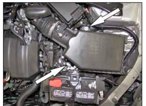
5. Loosen and remove the two bolts securing the factory air box.
