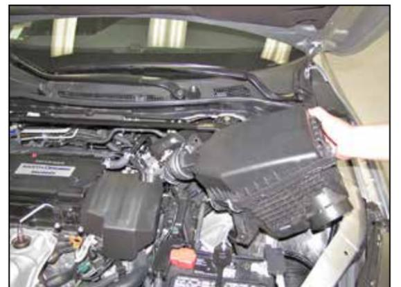
6. Remove the complete factory intake system from the vehicle.
