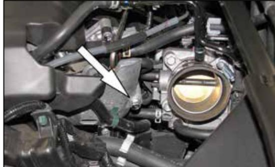
13. Remove the bolt shown from the engine; this bolt will be reused in the next step.
