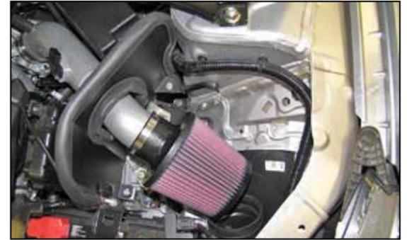
18. Install the K&N® air filter onto the K&N® intake tube and secure with the provided hose clamp
