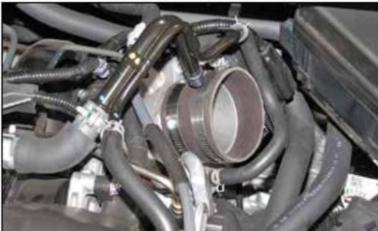
10. Install the provided silicone hose (084014) onto the throttle body and secure with the provided hose clamp.
