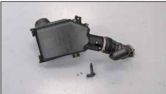
11. Remove the two screws securing the mass air sensor and then remove the mass air sensor from the vehicle.
