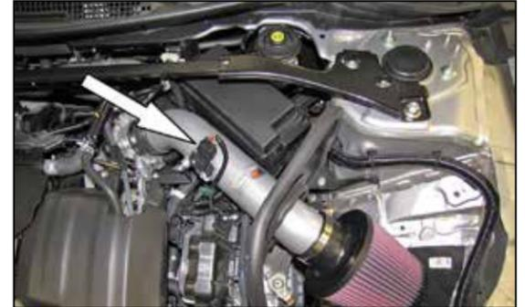
19. Reconnect the mass air sensor electrical connection.
