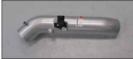
12. Install mass air sensor into the K&N® intake tube and secure with the provided hardware.
