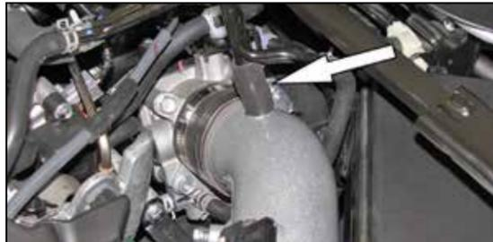
17. Connect the factory crank case vent pipe to the K&N® intake tube using the 1-1/2" long section of crank case vent hose from the previous step.
