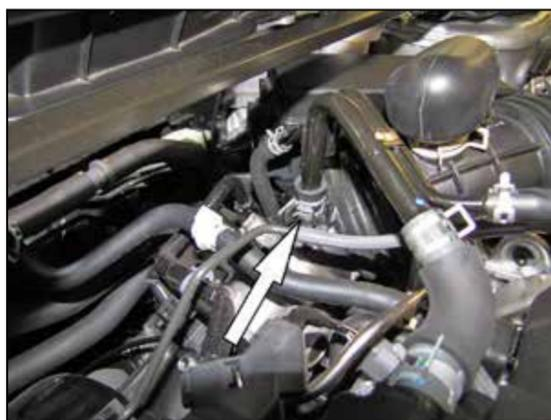
3. Release the spring clamp securing the crank case vent pipe to the factory intake tube and then disconnect the vent pipe from the intake tube.
