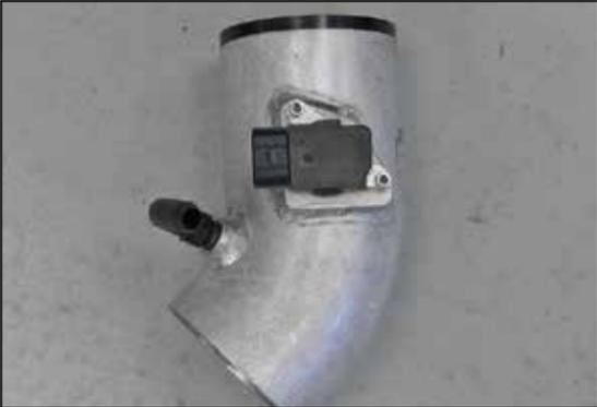
25. Install the mass air sensor into the K&N® intake tube and secure with the provided hardware.
