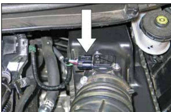
2. Disconnect the mass air sensor electrical connection and unhook the wiring harness from the upper air box.
