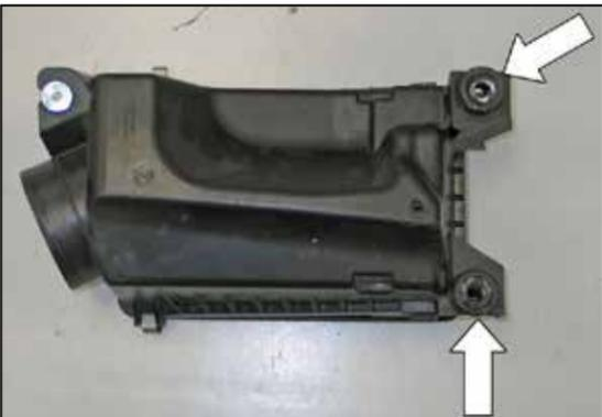
11. Remove the two mounting grommets shown from the factory lower air box.
