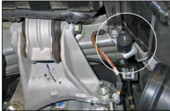
15. Install the provided rubber mounted stud onto the factory air box mounting location as shown.
