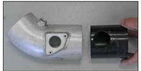
22. Install the venturi into the K&N® intake tube as shown.
