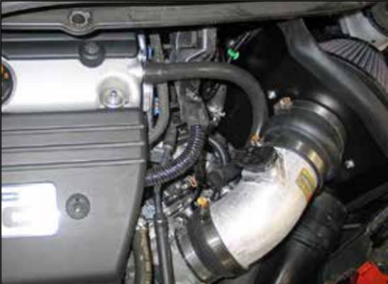
27. Install the provided silicone hose onto the 90° fitting attached to the K&N® intake tube. Attach the open end of the hose to the valve cover port as shown.
