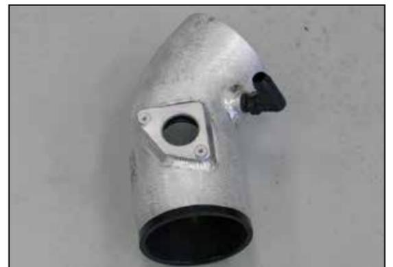
23. Install the provided 90° vent fitting into the K&N® intake tube as shown.
