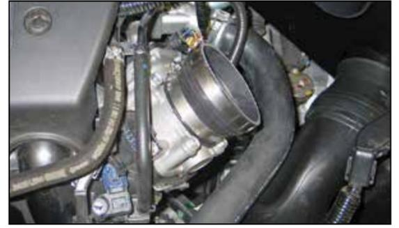
18. Install the provided silicone hose (084034) onto the throttle body and secure with the provided hose clamp.
