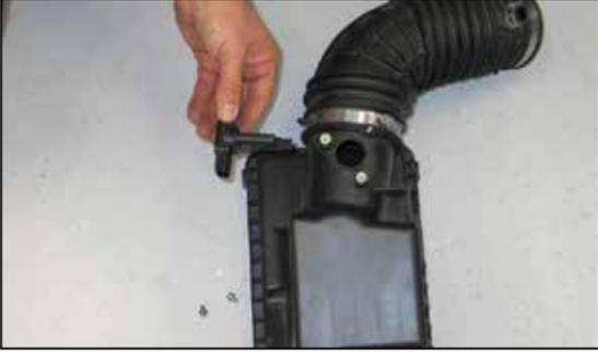
24. Remove the two screws securing the mass air sensor into the factory air box, then remove the sensor from the air box.
