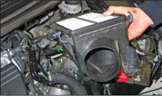
7. Lift up the front of the air box and disconnect the fresh air intake tube, then dislodge the air box from the mounting grommets and remove the air box from the vehicle.
