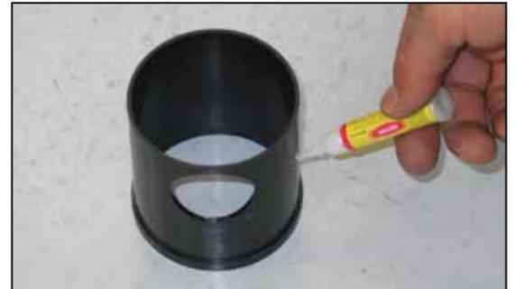
21. Apply several drops of the provided "Super Glue" to the lip of the venturi as shown.
