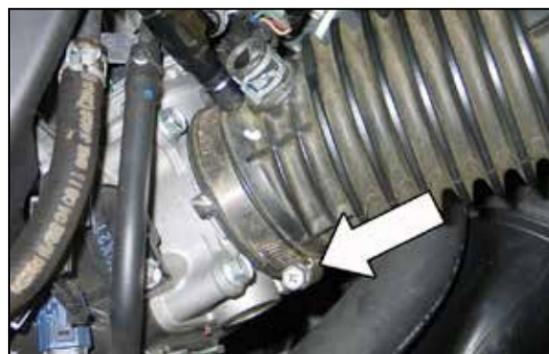
4. Loosen the hose clamp securing the intake tube to the throttle body.
