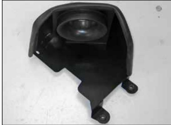
14. Install the filter adapter into the heat shield and secure with the provided hardware.
