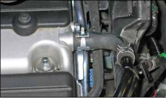
9. Release the spring clamp securing the crank case vent hose to the valve cover and then disconnect the hose from the valve cover.
