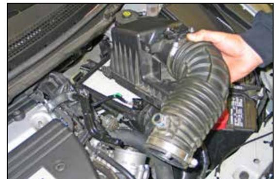
5. Release the two clips securing the upper air box to the lower air box and then remove the upper air box and intake tube assembly.
