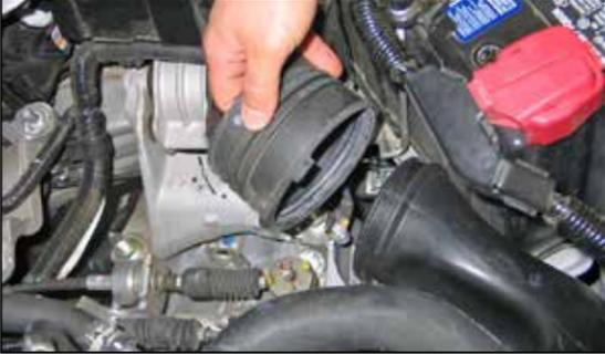
8. Remove the fresh air tube coupler as shown.
