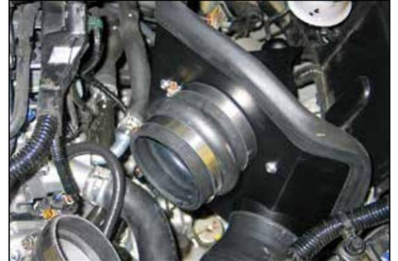
19. Install the provided silicone hose (5-576) onto the filter adapter and secure with the provided hose clamp.
