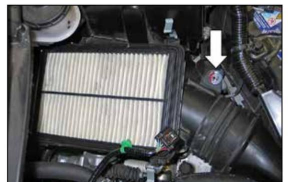
6. Remove the lower air box retaining bolt shown.
