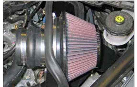
20. Install the K&N® air filter and secure with the provided hose clamp.
