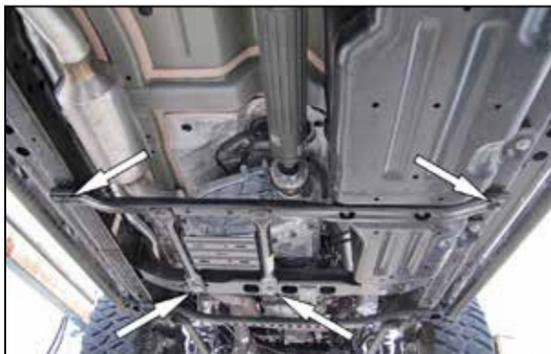
6. Remove the four bolts that secure the transfer case skid plate and the remove the skid plate from the vehicle.
