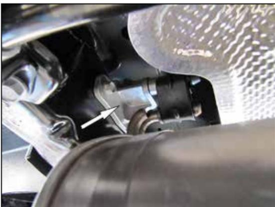
3. Loosen and remove the two bolts that secure the driver side muffer hanger to the chassis.
