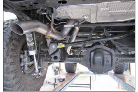
16. Check alignment and reposition as necessary. Once final position is satisfactory, tighten all band clamps from front to rear of vehicle.
