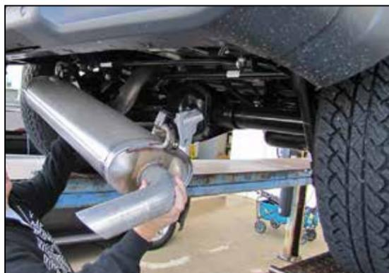
5. Using a twisting motion so the muffer pipe slides off the exhaust pipe, remove the muffer assembly from the vehicle.
