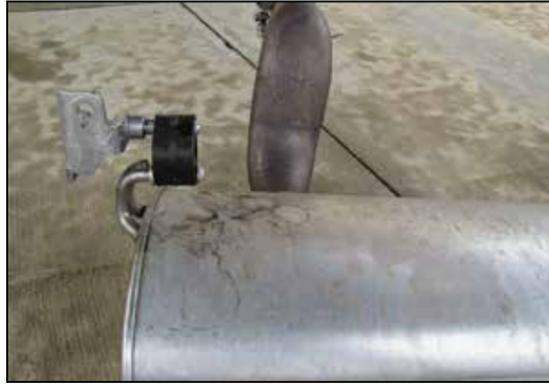
13. Remove the driver side muffer hanger from the stock muffer.
