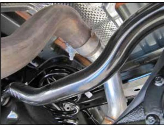
2. Loosen the clamp that secures the muffer pipe to the exhaust pipe.
