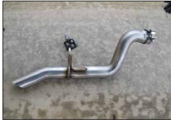
14. Install the driver side muffer hanger onto the K&N® tail pipe hanger.
