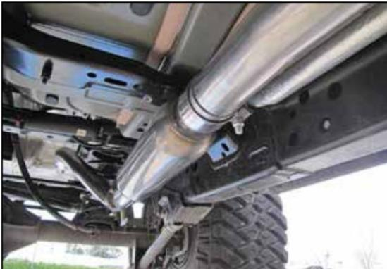
12. Install the K&N® muffer onto the K&N® mid pipe and into the factory hanger.
