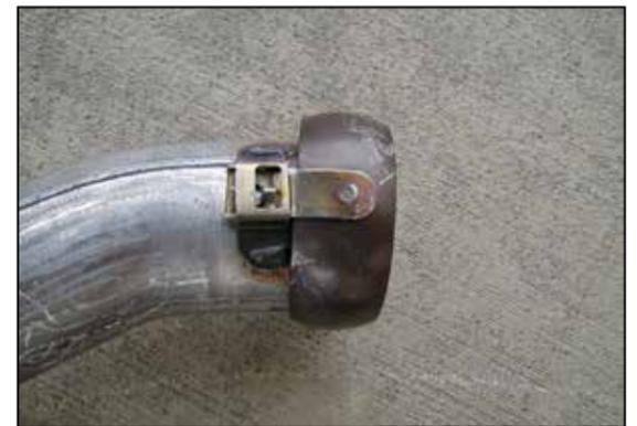
9. Release the locking tab and then remove the factory clamp from the exhaust pipe.
