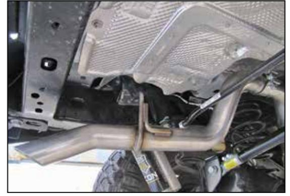
15. Install the K&N® tail pipe onto the K&N® exhaust pipe.
