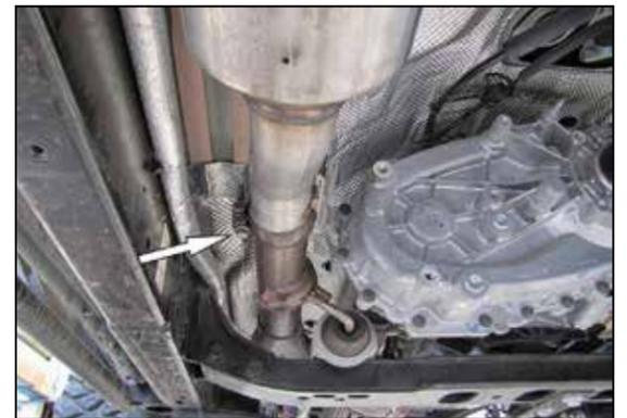
7. Loosen the clamp the secures the exhaust mid pipe to the exhaust catalyst pipe.
