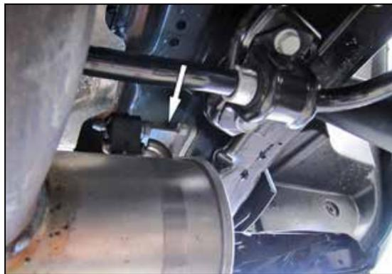
4. Loosen and remove the two bolts that secure the passenger side muffer hanger to the chassis.
