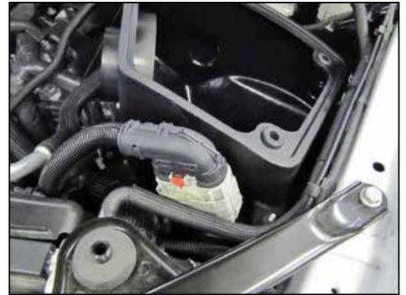
16. Clip the wiring harness onto the bracket installed onto the K&N® air filter housing.
