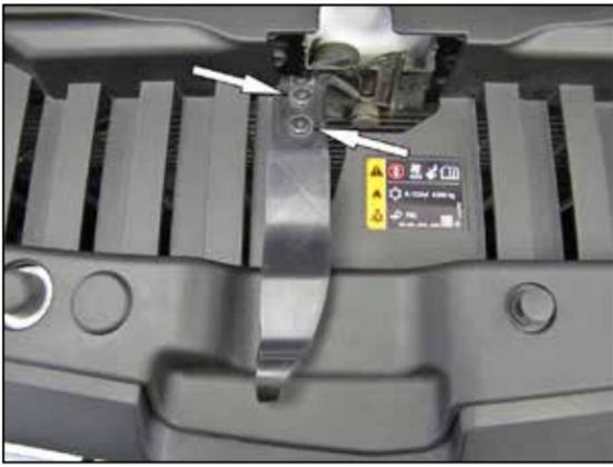
5. Remove the two bolts that secure the hood release arm to the hood latch and then remove the release arm.
