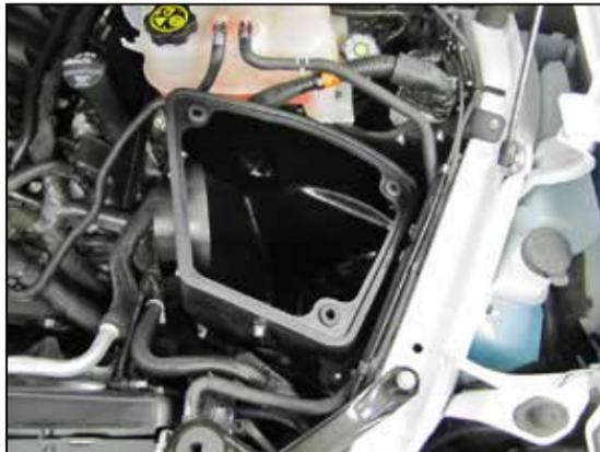
14. Install the K&N® air filter housing into the vehicle so the mounting grommets engage into the factory mounting holes. Secure the housing with the factory nut removed in step #9.
