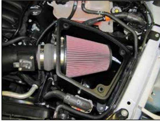
25. Install the K&N® air filter onto the filter adapter and secure with the provided hose clamp.
