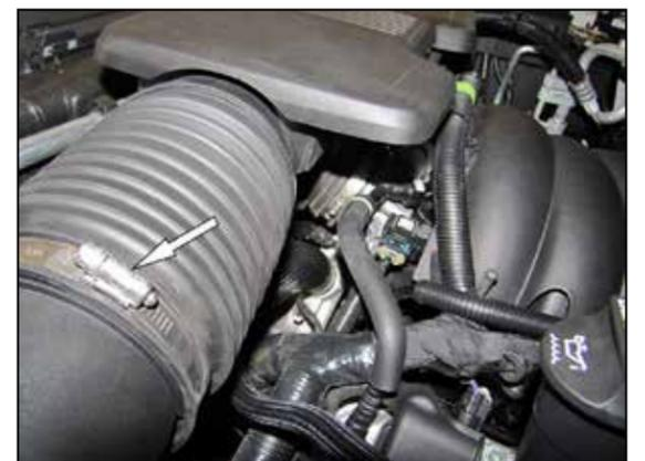
4. Loosen the hose clamps that secure the intake plenum assembly to the throttle body and air filter housing. Disconnect the plenum from the air filter housing and then rotate the plenum assembly counter clockwise to disengage the keyed mount and then remove the plenum from the throttle body.
