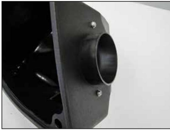
10. Install the provided radius filter adapter into the K&N® air filter housing and secure with the provided hardware.
