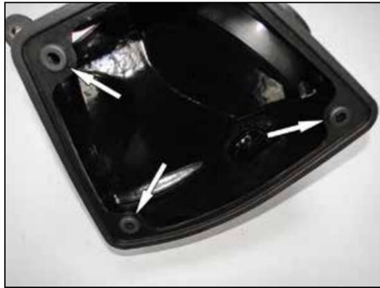
11. Install the three provided grommets into the top of the K&N® air filter housing.
