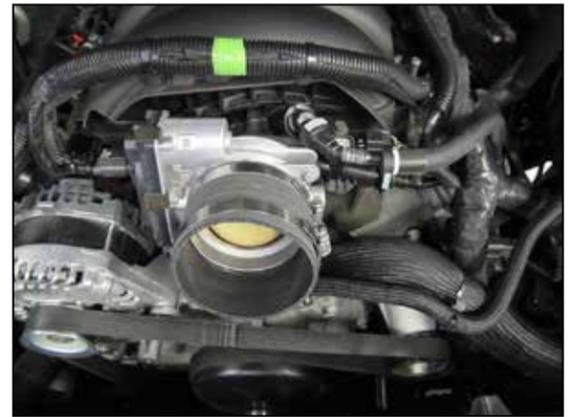
18. On 5.3L vehicles, install coupler #08497 onto the throttle body and secure with the provided hose clamp. On 6.2L vehicles, install coupler #084107 onto the throttle body and secure with the provided hose clamp.
