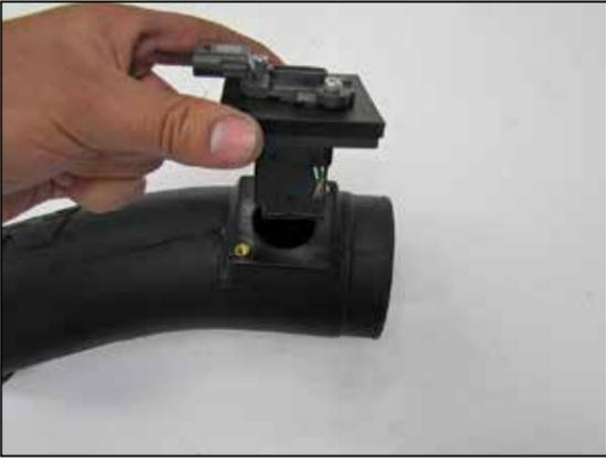
20. Install the mass air sensor assembly into the K&N® intake tube in the direction shown and secure with the provided hardware.
