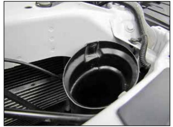
15. Push the factory fresh air intake duct into the K&N® air filter housing and then reinstall the plastic clip to secure it into position.
