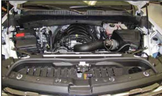
28. Reinstall the upper radiator valence and secure with the factory retaining clips.
