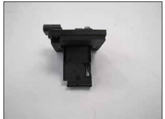
19. Install the provided gasket onto the provided mass air sensor adapter. Remove the mass air sensor from the factory air filter housing and then install it into the adapter and secure with the provide hardware.
