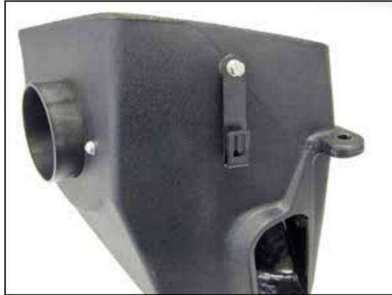
12. Install the provided wiring harness bracket onto the K&N® air filter housing and secure with the provided hardware.
