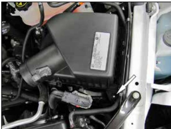
9. Remove the nut that secures the air filter housing assembly to the vehicle. Remove the air filter housing assembly from the vehicle.
