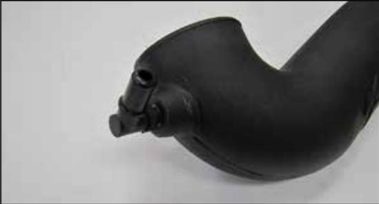
21. Install the 90° quick disconnect vent fitting into the K&N® intake tube as shown.
