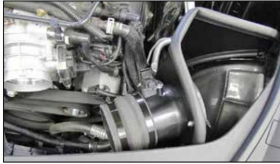
14. Install the provided hump coupler hose (084101) onto the mass air sensor housing and secure with the provided hose clamp.
