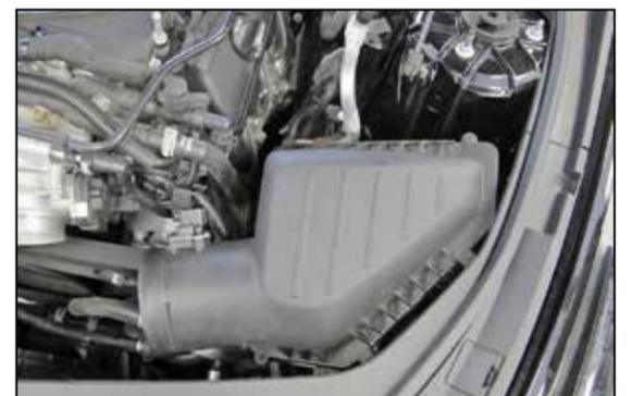
6. Lift the air filter housing assembly and remove it from the vehicle.
