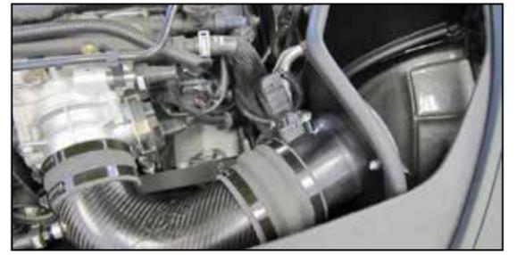
19. Connect the mass air sensor electrical connection.
