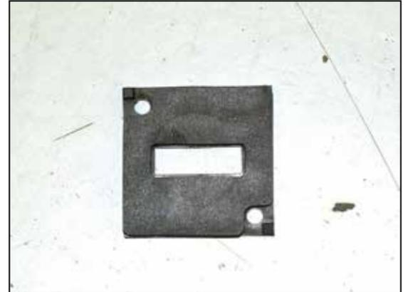
18. Install the provided gasket onto the K&N® mass air sensor adapter.
