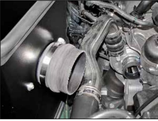
22. Install the provided hump coupler (08699) onto the filter adapter and secure with the provided hose clamp.
