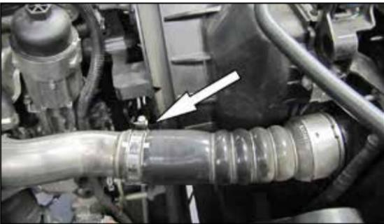
9. Loosen the charge tube flex hose and rotate it inwards 90° as shown and then retighten the clamp.
