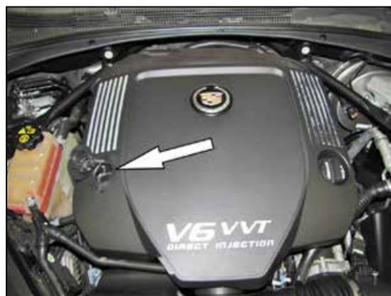
3. Lift up the small cover on the decorative engine cover to gain access to the bolt securing the cover. Remove the bolt securing the cover, remove the oil cap and then remove the decorative engine cover. Reinstall the oil cap.
