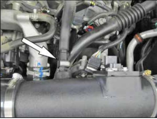
23. Connect the crank case vent hose to the quick disconnect fitting installed into the K&N® intake tube.
