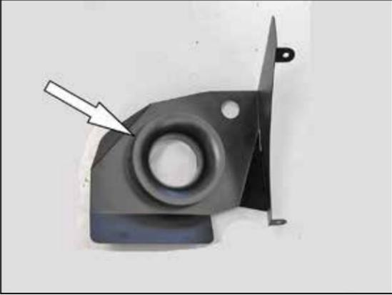
8. Install the filter adapter into the K&N® heat shield and secure with the provided hardware.
