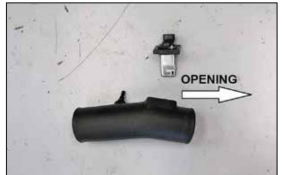
20. Install the mass air sensor assembly into the K&N® intake tube; be sure to install the sensor in the correct direction.
