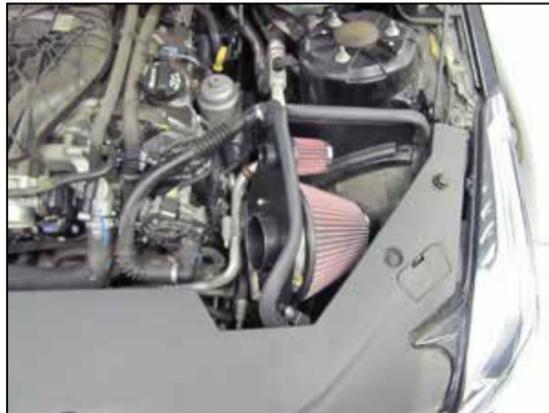
15. Install the heat shield assembly into the vehicle so that the mounting studs insert into the mounting grommets, then secure the mounting bracket to the core support. Tighten all of the hardware securing the heat shield.
