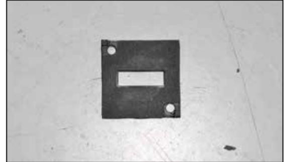
17. Install the provided gasket onto the mass air sensor adapter.
