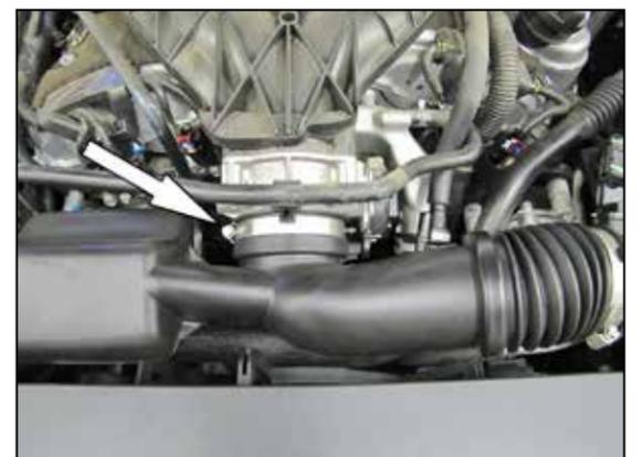
6. Loosen the hose clamp securing the intake tube to the throttle body. Disconnect the factory intake tube from the throttle body.
