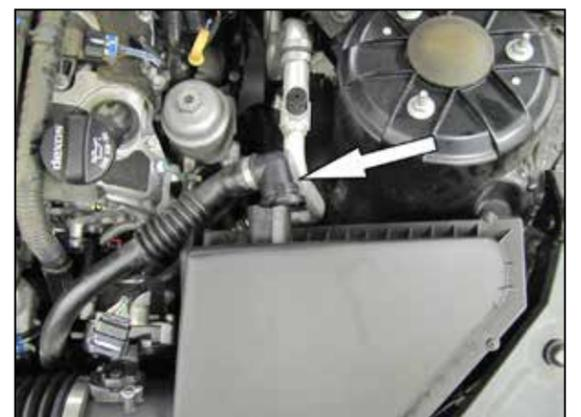
5. Release the air injection quick disconnect fitting and then disconnect the air injection tube from the factory air box.
