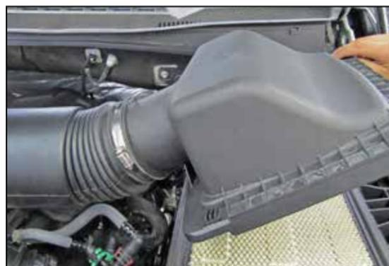
4. Release the locking clips that secure the upper air filter housing to the lower housing, then lift the upper housing and remove it from the vehicle. Remove the factory air filter from the vehicle.
