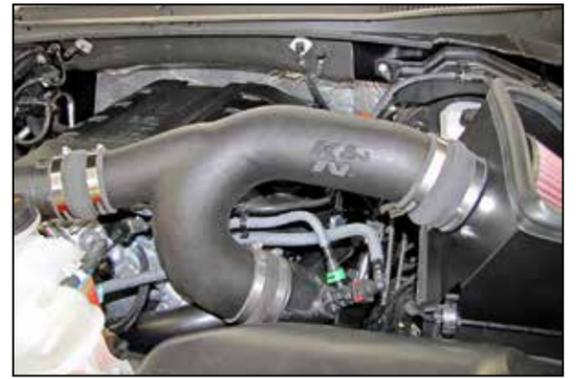
17. Install the K&N® intake tube into the couplers at the turbo inlet tubes and then into the coupler at the filter adapter, adjust the tubes for best fit and then secure with the provided hose clamps.
