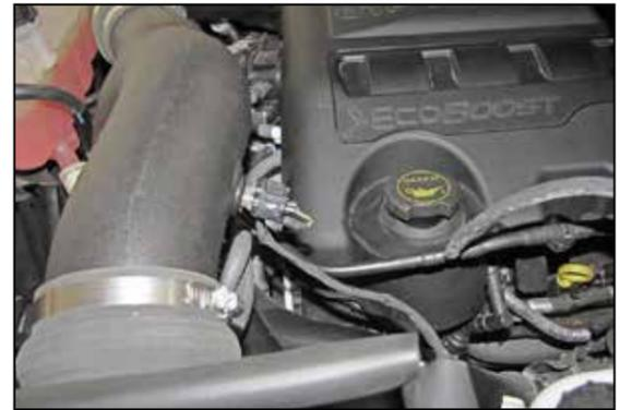
18. Reconnect the inlet air temperature sensor electrical connection using the provided extension harness.
