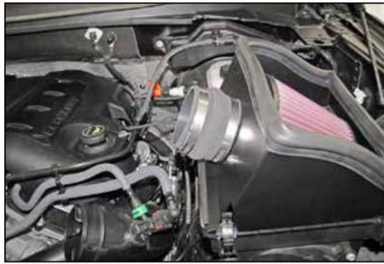
12. Install the provided hump coupler (08699) onto the filter adapter and secure with the provided hose clamp.
