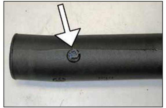
20. Install the inlet air temperature sensor into the K&N® intake tube.
