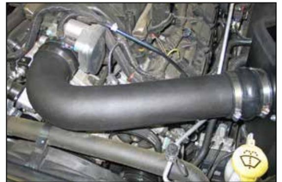
21. Install the K&N® intake tube into the hump hose at the filter adapter and then into the hose at the throttle body. Adjust the tube and heat shield for best fit and clearance and then secure with the provided hose clamps
