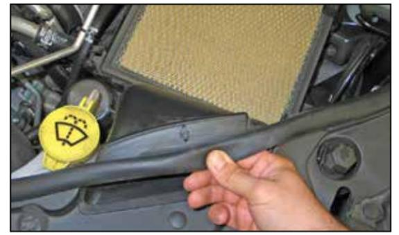
8. Unhook the sealing trim from the fresh air intake scoop.
