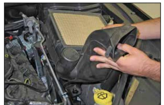
9. Lift up the lower airbox to dislodge it from the mounting grommets and then remove the lower airbox from the vehicle. Some vehicles may have a power steering line attached to the air box than will need to be unhooked.
