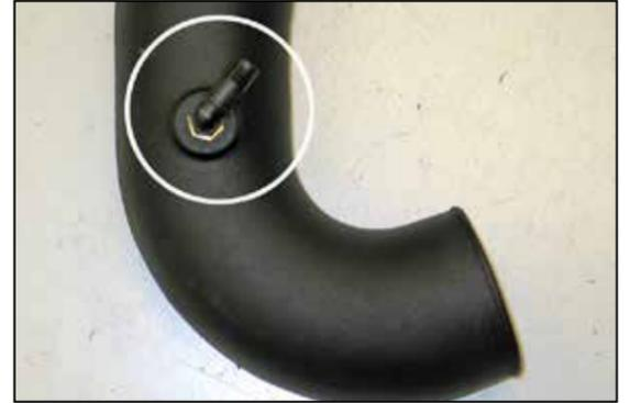
21. Install the 90° npt fitting into the K&N® intake tube as shown.
