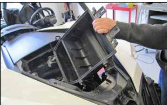
11. Have an assistant lift up the front of the body work, then pull the air filter housing forward and disconnect the intake tube from the throttle body. Rotate the air filter housing counter clockwise 90° and guide it out through the opening in the body work to remove it from the vehicle.
