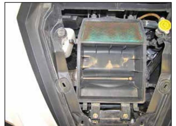
5. Release the clips which secure the upper air filter housing and then remove the upper air filter housing and air filter.
