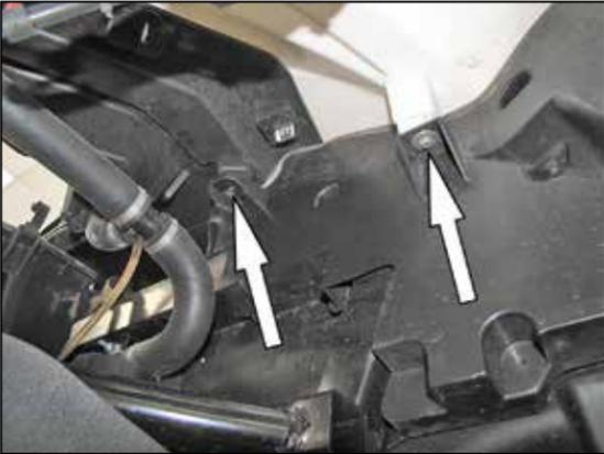
9. Remove the four bolts securing the front body work.
