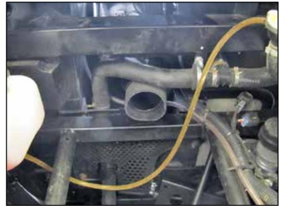
16. Install the provided hump coupler (08439) onto the K&N® intake tube and secure with the provided hose clamp.
