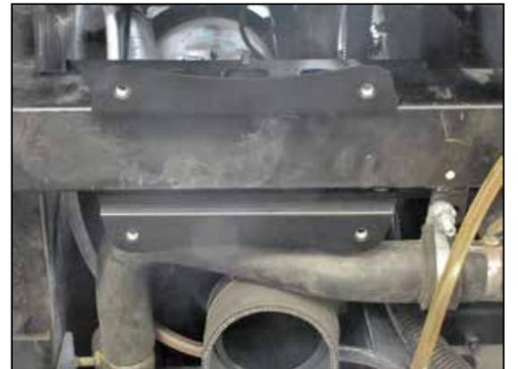
18. Install the K&N® air filter box mount over the frame cross member.
