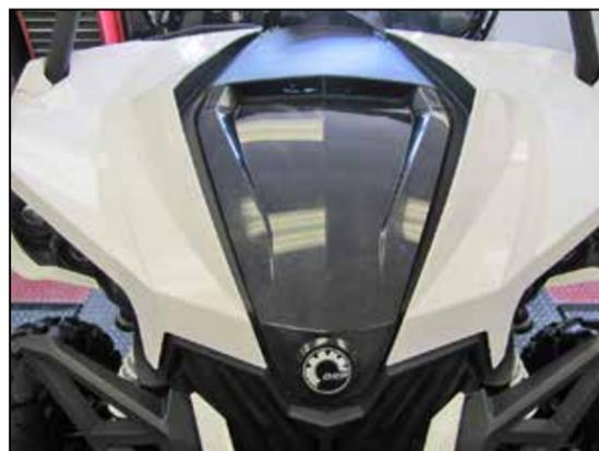
4. Remove the hood panel to access the air filter housing.
