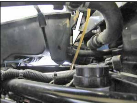
10. Reach through the driver's side wheel opening and locate the crank case vent hose attached the rear of the air filter housing. Release the spring clamp and disconnect the crank case vent hose from the air filter housing.
