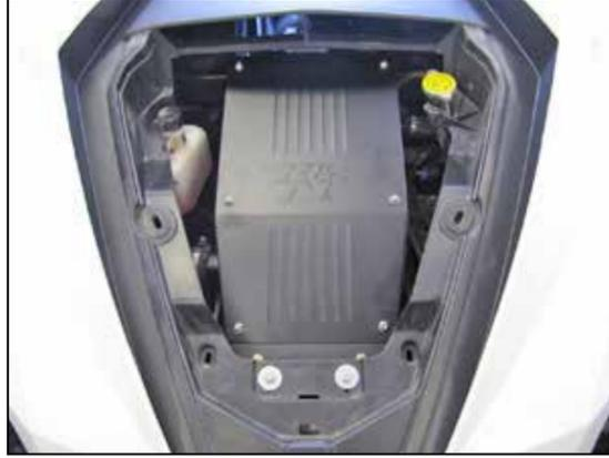
25. Install the K&N® air box lid and secure with the provided hardware.
