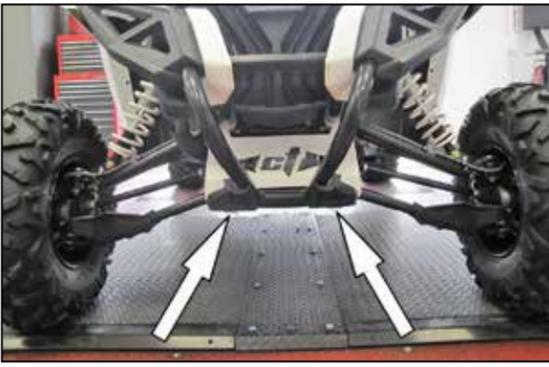
7. Remove the upper bumper bolts, remove the lower plastic bumper covers and then loosen the lower bumper bolt. Swing the bumper down/forward.
