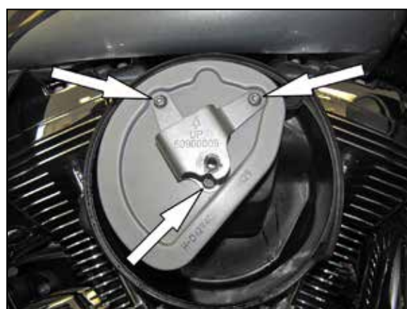
4. Remove the three bolts which secure the factory air filter to the base plate and then remove the air filter from the vehicle.
