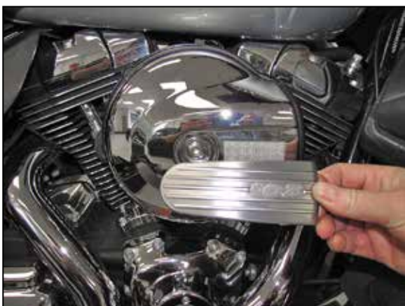
2. Remove the decorative badge from the air filter cover.
