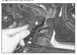
13. Fit the 'L' bracket supplied to the stud located on the original air box support frame & secure using the original nut previously removed as shown.
