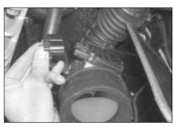
22. Reconnect the electrical harness plug from the MAS (Mass Air Sensor).
