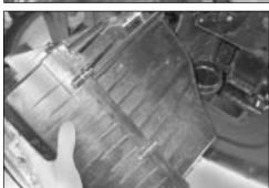
8. Unclip & remove the intake hose from the air box assembly & carefully remove the assembly from the vehicle.
