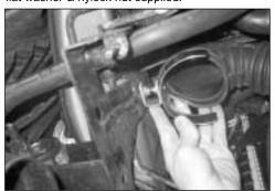
12. Fit the mounting bracket assembly to the original air box support frame & secure using the original bolt as shown.
