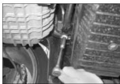
4. Remove the 4 bolts securing the air box assembly to the vehicle (You may wish to remove the battery / battery tray to gain access to the upper bolts).
