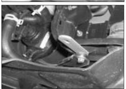
14. Remove the bolt securing the bottom of the original air box support frame. Slide the 'Flat' bracket supplied between the support frame & lower support. Secure the bracket using the original bolt.
