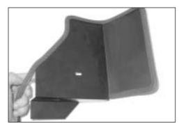
15. Fit the edge trim to the heat shield as shown. Remove any excess trim if necessary
