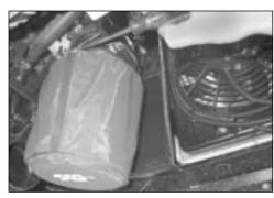
24. Slide the new filtercharger onto the rubber filter adaptor & tighten the #64 hose clip supplied.
