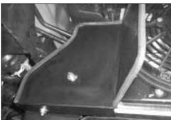
16. Attach the heat shield supplied to the 'L' & 'Flat' brackets. Secure the shield in place using the bolts, washers & nylock nuts supplied.
