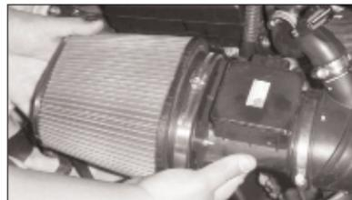
12. Install the Filtercharger assembly into the intake tube.
