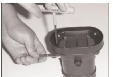
9. Attach the adapter to the mass air sensor and secure it using the hardware provided.
