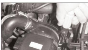
4. Loosen the hose clamp at the intake tube.
