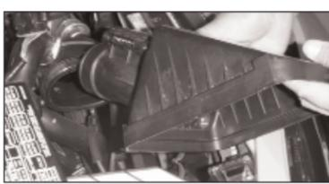
5. Unclip the airbox top and remove the complete airbox top assembly.
