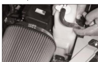
16. Slide the coolant reservoir tank back onto its retaining bracket.
