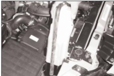
3. Slide the coolant reservoir tank up off its retaining bracket and set it aside.
