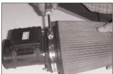
10. Attach the Filtercharger element onto the adapter and secure it with the provided hose clamp.
