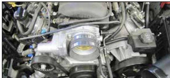
15. Install the provided coupling hose (08761) onto the throttle body and secure with the provided hose clamp.
