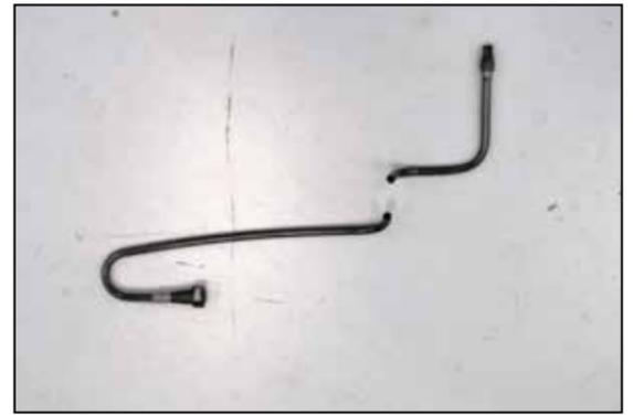
18a. On 2014 and later vehicles, it will be necessary to cut the crank case vent tube as shown. Then connect the Cut section of tube to the oil filler cap. Attach the supplied hose to the to the trimmed section of crank case vent tube,
