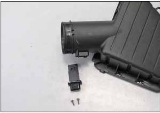
7. Remove the mass air sensor from the air filter cover.
