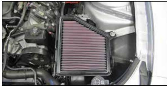
13. Remove the factory air filter and replace with the provided K&N® air filter.
