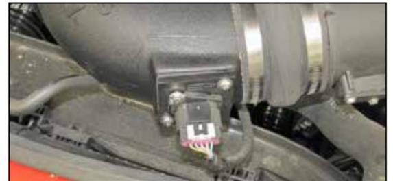
19. Reconnect the mass air sensor electrical connection.
