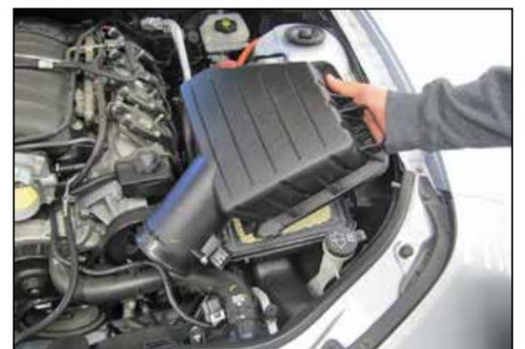
6. Release the two clips securing the air filter cover and then remove the air filter cover.
