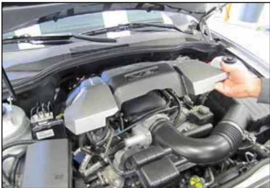
2. Remove the oil cap and then lift off the engine cover. Reinstall the oil cap.
