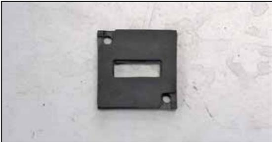
9. Install the provided gasket onto the K&N® mass air sensor adapter.
