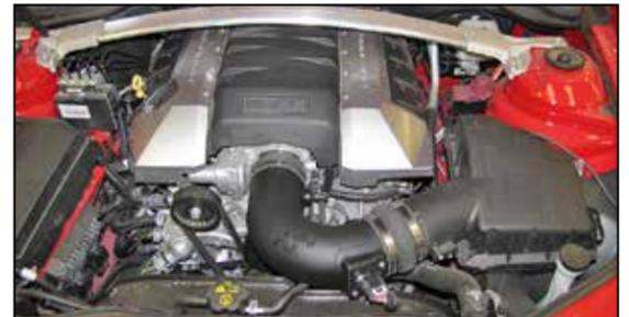
20. Reinstall the engine cover, Reconnect the negative battery cable. Double check to make sure everything is tight and properly positioned before starting the vehicle.
