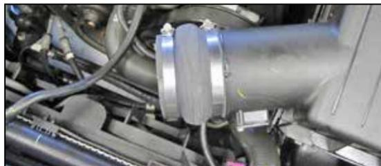
16. Install the provided coupling hose (08418) onto the air filter cover and secure with the provided hose clamp.
