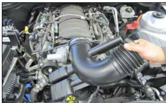
4. Loosen the clamps securing the intake tube to the throttle body and air filter housing and then remove the factory intake tube.
