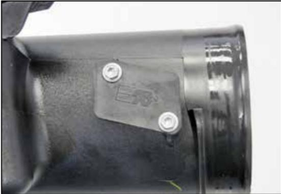
8. Using the factory screws from the previous step, install the mass air sensor block off plate and gasket.
