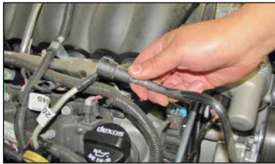
3. Disconnect the crank case vent tube from the valve cover port.
