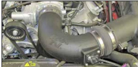
17. Install K&N® intake tube into the hose at the throttle body and then into the hose at the air filter cover, adjust the tube for proper fit and then secure with the provided hose clamps.
