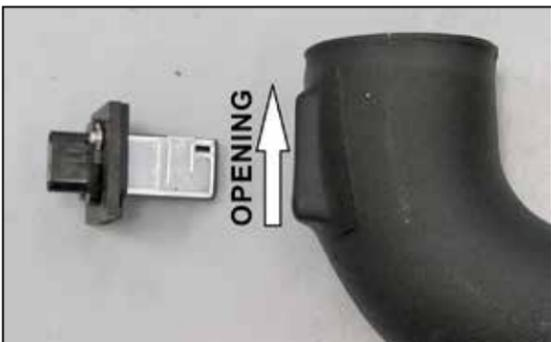
11. Install the mass air sensor assembly into the K&N® intake tube so the opening is pointed towards the air filter end of the tube and secure with the provided hardware.
