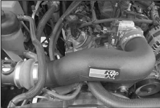
21. Install the K&N® intake tube into the silicone hose at the throttle body and mass air sensor and secure with the provided hose clamps.
