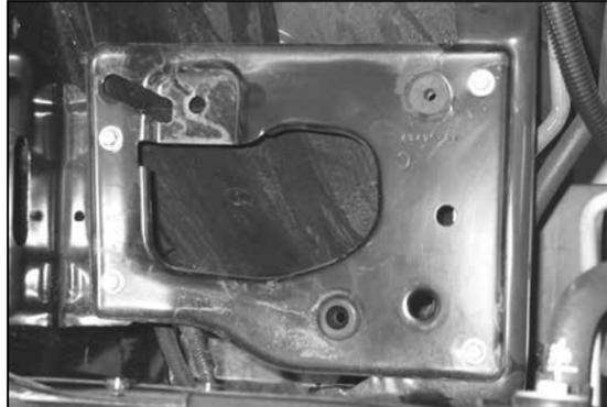
11b. Remove the heat shield assembly and drill a 5/8" hole through the marked location from step #11a.
