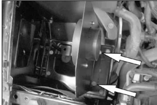
13. Install the heat shield assembly onto the airbox mounting tray and secure to the 5/16" inserted nuts with the provided hardware as shown.
