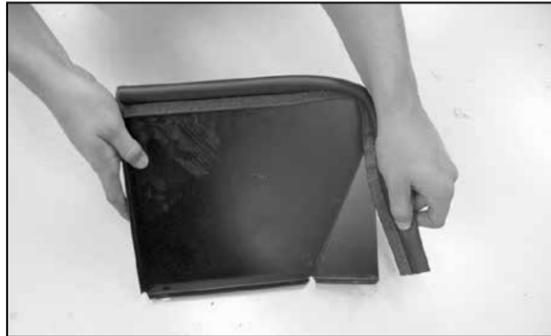
25. Install the provided edge trim onto the filter cover as shown.
