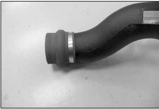
20. Install the silicone hump hose (08543) onto the K&N® intake tube and secure with the provided hose clamp as shown.
