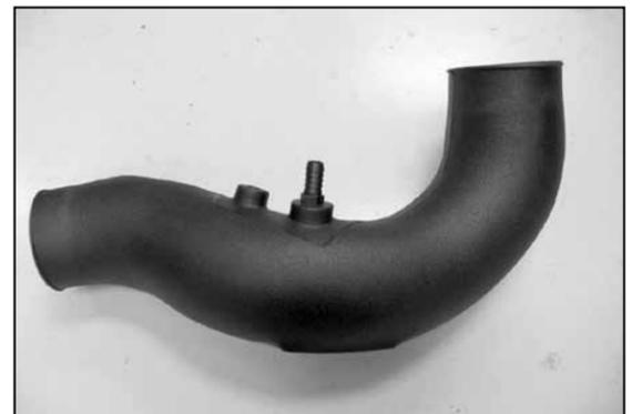
18. Install the NPT fitting into the K&N® intake tube as shown.
