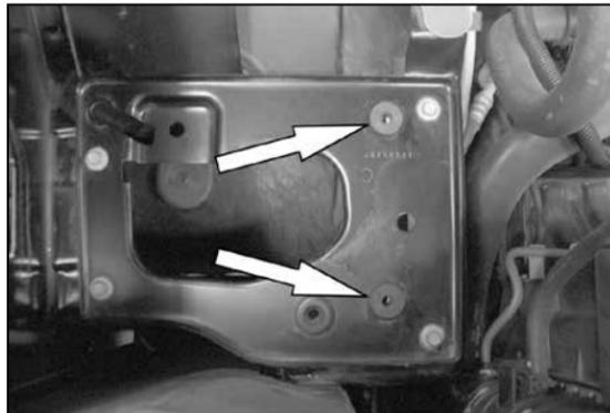
12. Install the two 5/16" inserted nuts into the airbox mounting tray as shown.
