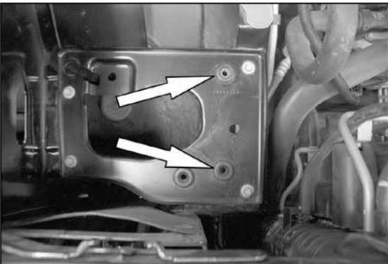
11. Remove the two airbox mounting grommets shown.
