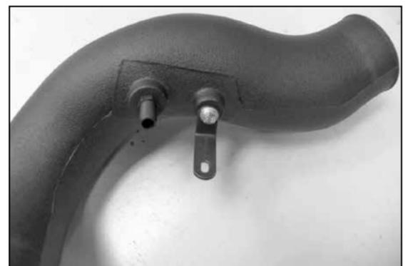
19. Install the "L" bracket (070812) onto the K&N® intake tube with the provided hardware as shown.
