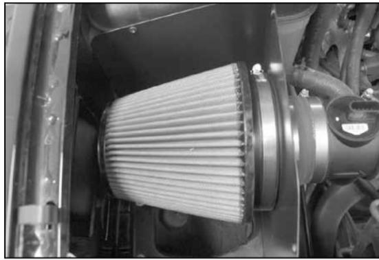
24. Install the K&N® air filter as shown and secure with the provided hose clamp.
