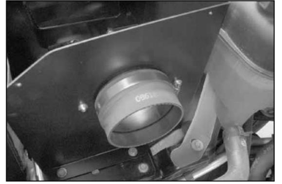
15. Install the silicone hose (08618) onto the filter adapter and secure with the provided hose clamp.
