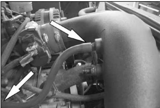
23. Install the provided crankcase vent hose onto the valve cover and then onto the K&N® intake tube as shown.
