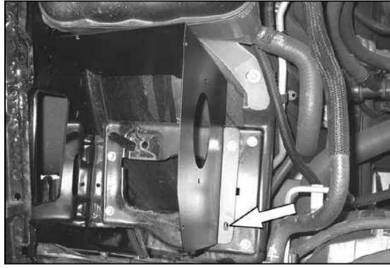
11a. On vehicles that are not equipped with the front airbox mounting grommet and hole, install the heat shield assembly as shown. Then, use a marker to mark the mounting plate through the heat shield mounting hole.
