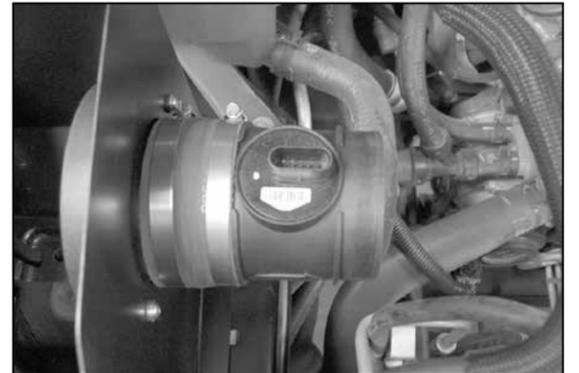
17. Install the mass air sensor assembly into the silicone hose on the filter adapter and secure with provided hose clamp.
