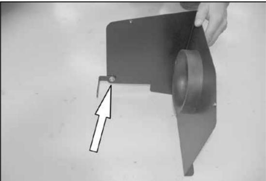
10. Install the "L" bracket (010031) onto the heat shield with the provided hardware as shown.
