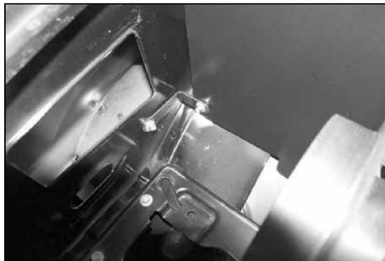
14. Secure the heat shield mounting bracket to the inner fender with the fender washers and hardware as shown.
