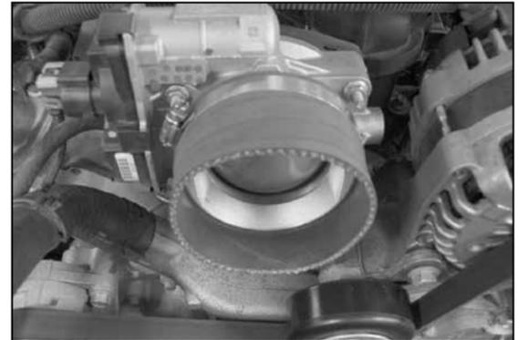
16. Install the silicone (08631) hose onto the throttle body and secure with the provided hose clamp.
