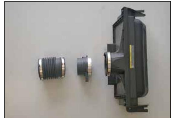
8. Loosen the two hose clamps securing the mass air sensor to the stock air box and intake tube, and then remove the mass air sensor.
