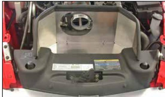
17. Reinstall the core support cover removed in step #5 and secure with the retaining clips removed step #3 and the factory nuts removed in step #4.
