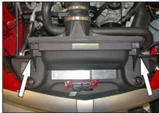
4. Remove the two 10mm nuts, which hold the core support cover onto the air box.
