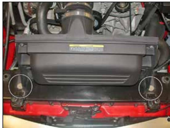
6. Remove the two bolts, which secure the air box to the core support.
