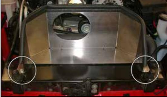
11. Install the heat shield assembly onto the air box mounting points and secure with the provided hardware.
