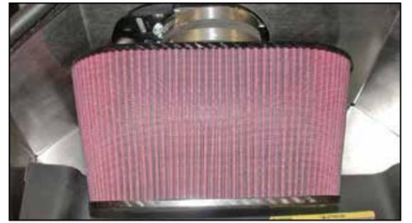
20. Install the air filter onto the mass air sensor and secure with the provided hose clamp.
