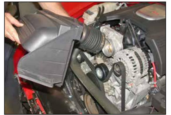
7. Loosen the hose clamp that secures the stock intake tube to the throttle body, and then remove the complete intake assembly from the vehicle.
