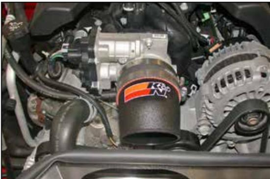
13. Install the K&N® intake tube into the silicone hose at the throttle body and secure with the provided hose clamp.
