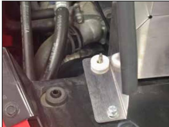
16. Install the two provided nylon spacers onto each side of the air box mounting studs as shown.
