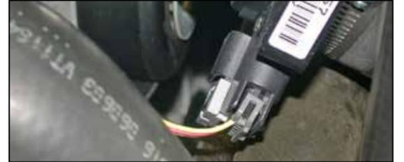
21. Reconnect the mass air sensor electrical connection.
