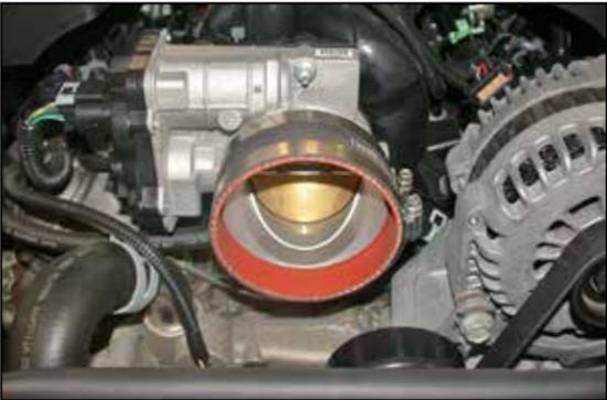
12. Install the provided silicone hose (08625) onto the throttle body and secure with the provided hose clamp as shown.
