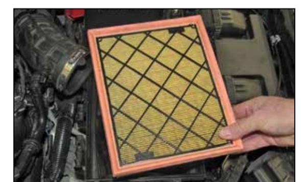
5. Release the two upper air box retaining clips and then remove the upper air box and stock air filter.
