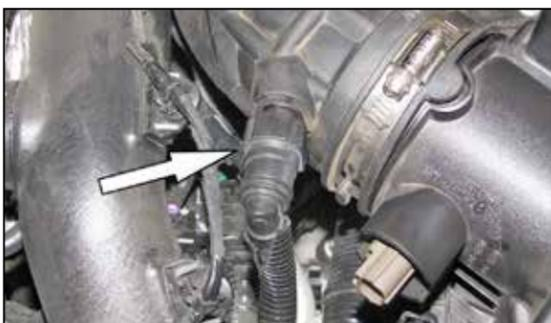
3. Disconnect the crank case vent connection.
