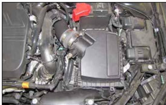
17. Install the upper air box and Intake tube and then secure the air box with the factory clips. Adjust the intake tube for best fit and then secure it with the hose clamps provided to the two hump hoses.
