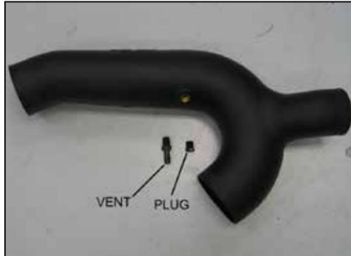
17. On vehicle equipped with an EVAP vent line, install the npt vent fitting into the K&N® intake tube. On vehicles not equipped with an EVAP vent line, install the npt plug.
