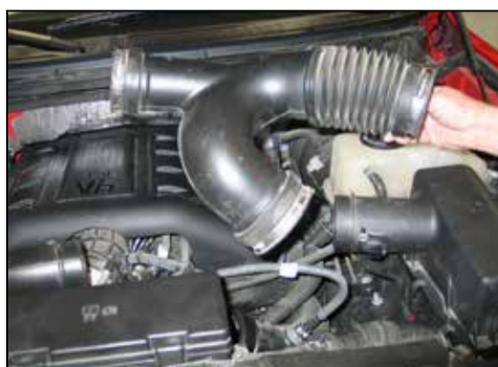
5. Remove the factory intake tube as shown. **NOTE: DO NOT remove the air diverters from the factory turbo inlet tubes.**
