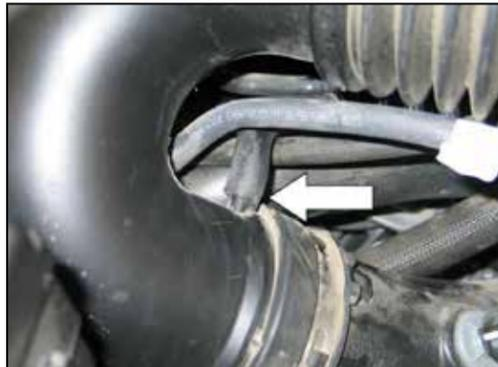
3. On vehicles equipped with the EVAP vent line, disconnect the EVAP vent line from the factory intake tube.
