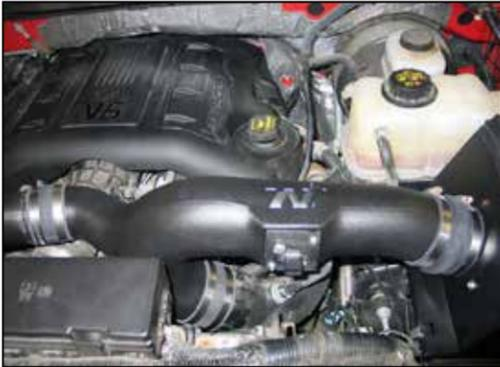
25. Install the K&N® intake tube assembly, attaching each inlet into the silicone hoses previously installed. Secure the intake tube with the provided hose clamps.
