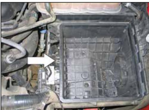
13. Remove the center upper air box retaining clip from the lower air box.
