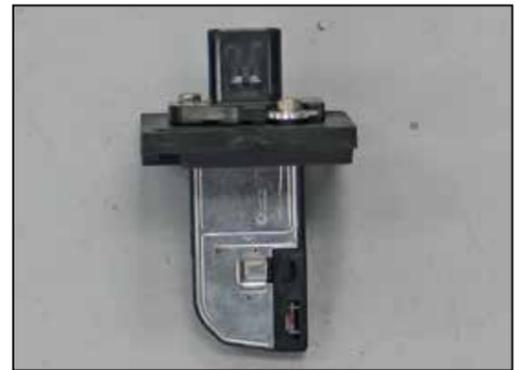
20. Install the mass air sensor into the mass air sensor adapter and secure with the provided hardware.
