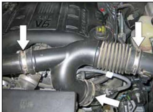
4. Loosen the three hose clamps securing the factory intake tube.
