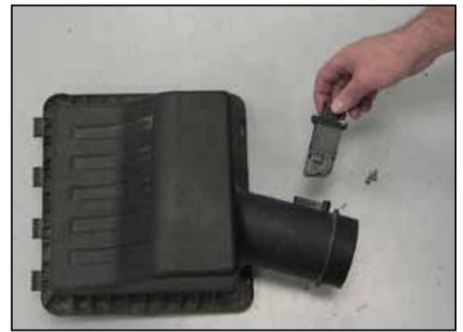
19. If the vehicle is equipped with a mass air sensor, remove the two bolts securing the mass air sensor into the factory air box and then remove the sensor from the air box.
