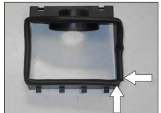
8. Install the provided "Top Bulb" edge trim around the top of the heat shield as shown. **NOTE: Some trimming of the edge trim will be necessary.**
