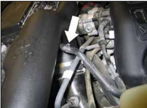
26. On vehicles equipped with an EVAP vent line, install the EVAP vent hose onto the vent fitting and secure with the provided hose clamp.
