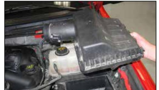
6. Release the three locking tabs and then lift up and remove the upper air box from the vehicle. **NOTE: K&N Engineering, Inc., recommends that customers do not discard factory air intake.**
