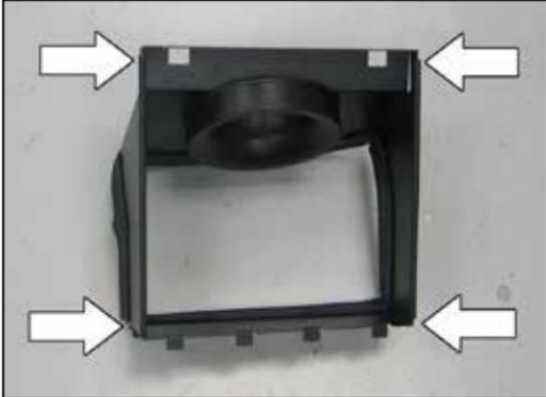
10. Install the 1/16" gap edge trim onto the bottom of the heat shield as shown.
