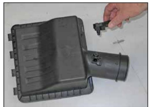
22. If the vehicle is equipped with a pressure sensor, remove the bolt securing the pressure sensor into the factory air box, and then remove the sensor from the air box.
