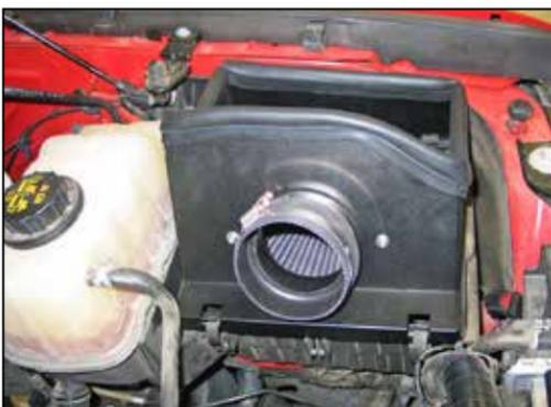
14. Install the air filter/heat shield assembly onto the lower air box and secure with the two remaining air box clips.
