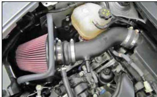
17. Install the K&N® intake tube into the coupler at the intake plenum and then slide the hump coupler onto the filter adapter. Adjust the intake tube for best fit and then secure with the provided hose clamps and heat shield mounting hardware.
