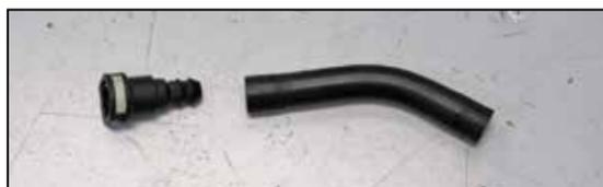
19. Remove the quick disconnect fitting from the factory flexible crank case vent line.
