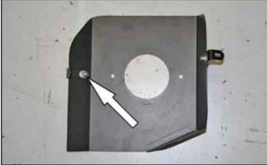
8. Install the heat shield mounting bracket (070712) onto the heat shield as shown using the provided hardware.
