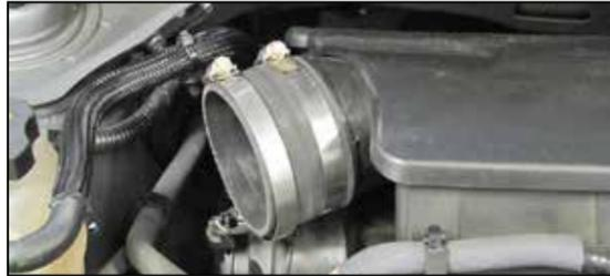
14. Install the provided coupler hose (08690) onto the intake plenum and secure with the provided hose clamp.
