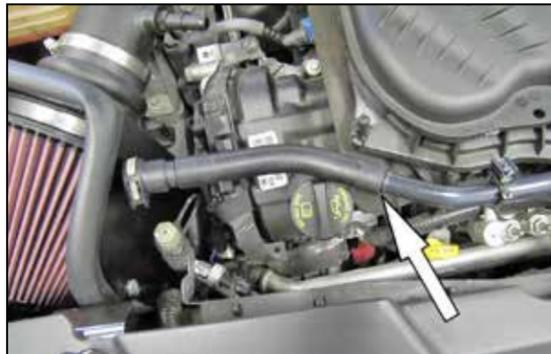
18. Remove the flexible crank case vent line from the hard line.
