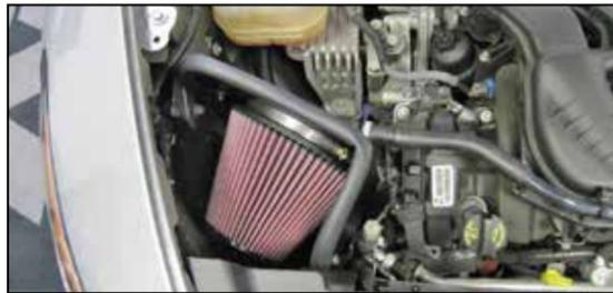
13. Install the heat shield assembly into the vehicle and secure with the hardware removed in step #6.
