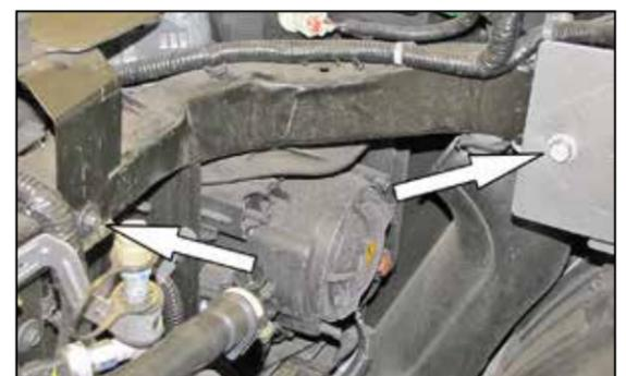
6. Remove the two factory bolts shown.
