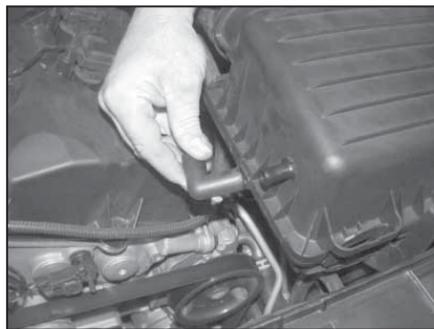
4. Disconnect the crank case vent hose from the airbox as shown.
