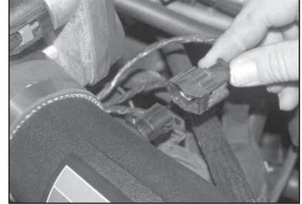
23. Reconnect the air temperature electrical connection as shown.
