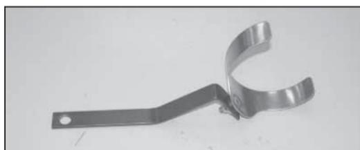
7. Assemble the tube-mounting bracket and saddle clamp as shown with the provided hardware.
