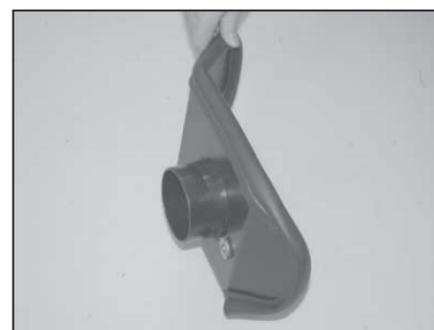
10. Install the air filter adapter onto the heat shield with the provided hardware as shown.
