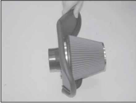
11. Install the K&N® air filter onto the filter adapter as shown.
