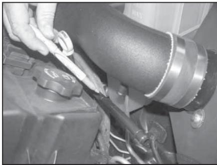
19. Mark the crank case vent tube approximately 1" back from the vent port on the K&N® intake tube as shown.
