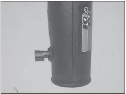
15. Install the air temperature sensor into the grommet installed in step #14.
