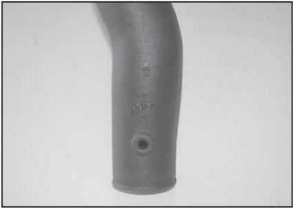
14. Install the grommet provide into the intake tube as shown.
