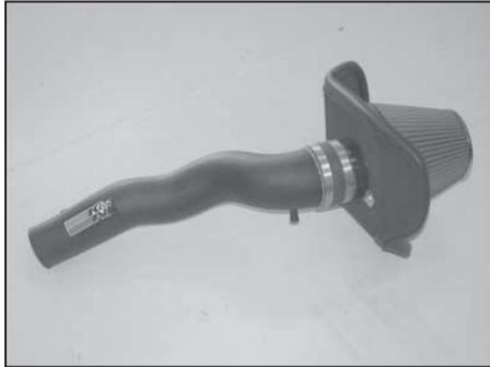
16. Install the air filter assembly onto the K&N® intake tube as shown.
