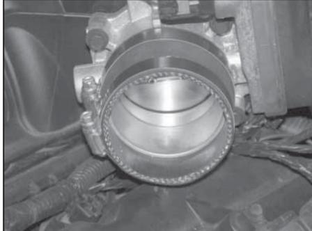
17. Install the silicone hose (08756) onto the throttle body and secure with the provided hose clamp as shown.
