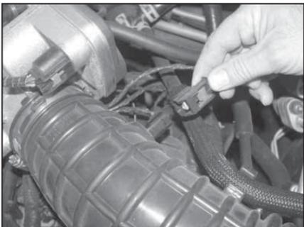
2. Unlock the red locking tab on the air temperature sensor electrical connection, then depress the locking lever and pull apart the air temperature sensor electrical connection.
