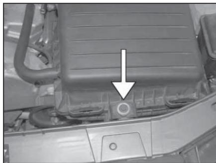
5. Loosen and remove the air box mounting bolt as shown.
