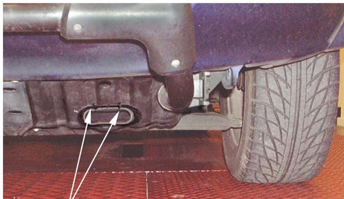
**1.** Taking all of the necessary safety precautions as per the manufacturers instructions, raise the front of the car. Unscrew and remove the L.H.S. undertray. Again taking all of the necessary safety precautions cut a rectangular hole in the undertray using the position and dimensions illustrated. Line the edge of the hole with the seal clip supplied (It may be necessary to trim the clip to suit the circumference of the hole)
