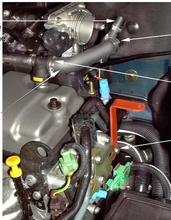
**3.** Insert half of the new plastic tube into the new breather hose and secure with a small hose clip supplied.
