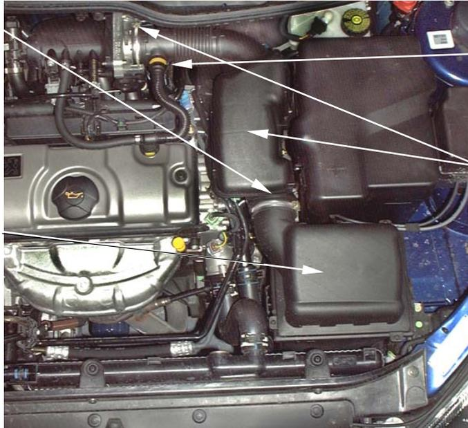
**3.** Remove the breather hose and IRV (Idle Regulator Valve) feed hose from the intake hose.
