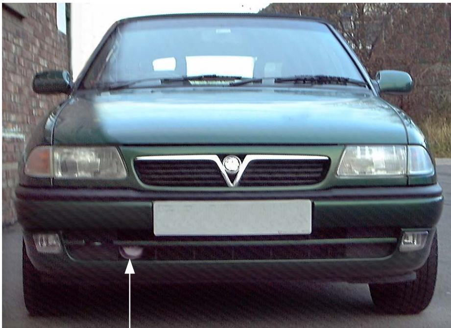
Feed the flexi cold air hose down to the front lower grille.
