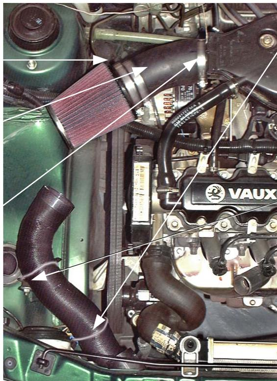
**5.** Carefully lengthen the flexi cold air hose to approx. 71cm / 28". Feed the hose down to the side of the radiator to the front lower grille. Drill / pierce a 3mm hole in the front air duct and tie the flexi cold air hose to it with a long plastic tie supplied. Ensuring that the hose clears the engine pulley.
