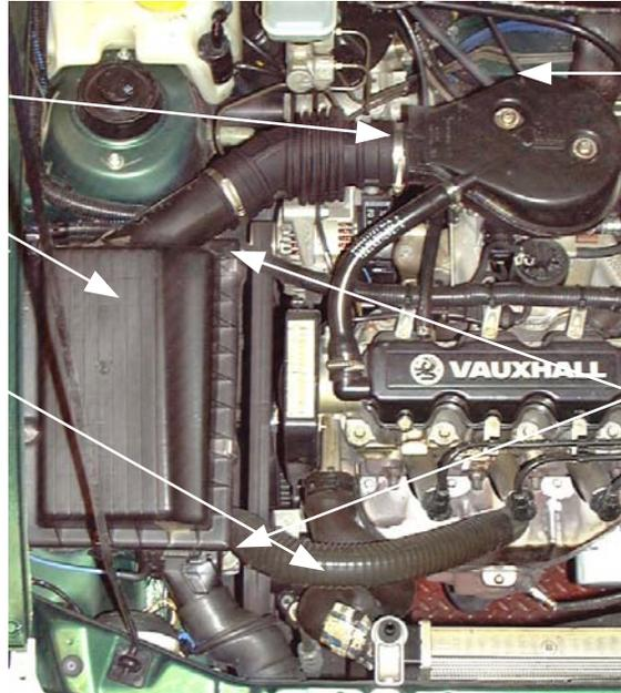
**4.** Remove the air box hot air flap vacuum hose from the rear of the intake housing. Blank off the vacuum outlet pipe with the rubber bung supplied.
